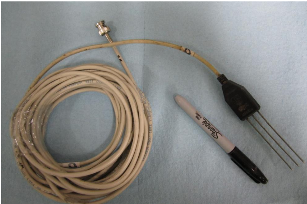
Figure 4.6. A typical CS640 TDR probe used in the column test
