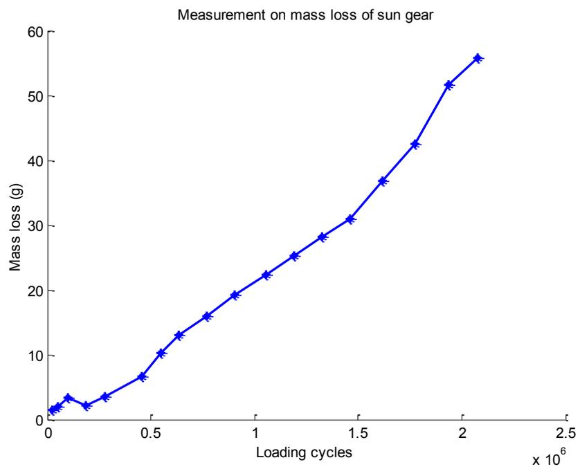
Figure 54. Measured mass loss of the sun gear
