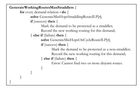
FIGURE 7.9. GenerateWorkingRoutesMaxStraddlers algorithm. Used to generate working routes for every demand relation such that the total number of potential straddling relationships is maximized.
