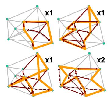
FIGURE 5.8. DRS based JCP FIPP *p*-cycle solution (corresponding to the second data point of the FIPP DRS JCP solutions in Figure 5.3).
