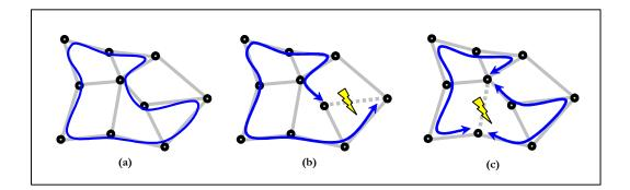
FIGURE 2.14. Example of (a) a *p*-cycle and the action taken after (b) an on-cycle and (c) straddling span failure.
