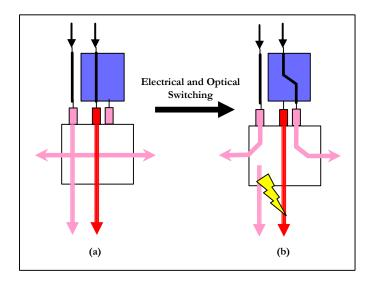
FIGURE 7.7. Implementation of an end-node of a straddling working route where one of the working paths is protected using same wavelength protection. (a) Pre-failure state. (b) Failure state.
