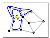
FIGURE 2.9. Span restoration example showing three replacement paths used to restore three units of working capacity affected by failure.
