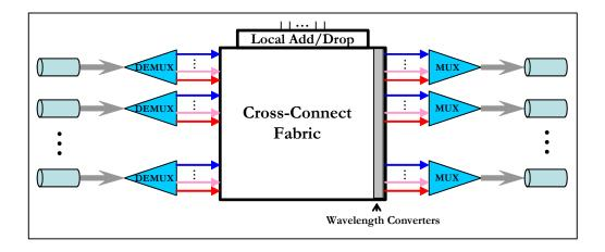
FIGURE 2.6. Optical cross connect (OXC).
