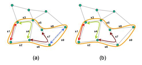
FIGURE 6.1. A four route DRS (arrowed lines) and the cycle originally generated to protect the DRS (solid thick connected line). The dashed arrowed line represents the over protected working path. (b) A possible outcome of actual protection assignment.
