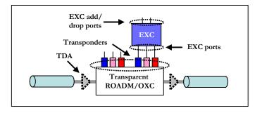
FIGURE 7.4. Generalized node model. Bidirectional schematic shown.
