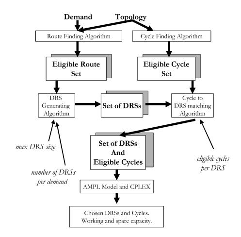
FIGURE 4.2. FIPP *p*-cycle DRS method.
