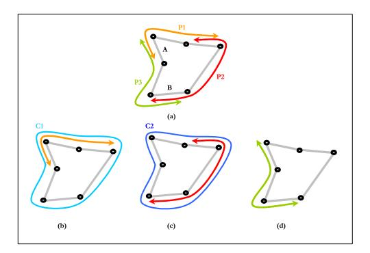
FIGURE 3.6. Path-protecting *p*-cycle example. a) Path set to be protected. b,c) Two cycles C1 and C2 assigned to protect the first two paths P1 and P2 respectively. c) P3 cannot be assigned a cycle for protection prior to failure.
