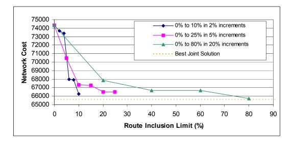
FIGURE 5.6. Network cost vs. eligible route inclusion threshold with DRS history propagation. The best joint solution refers to the FIPP DRS JCP data point corresponding to 2 eligible routes per demand in Figure 5.3.
