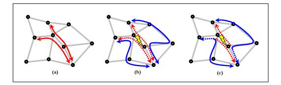
FIGURE 2.10. Path restoration single failure example: (a) Two working paths prior to failure. (b) PR without stub release. (c) PR with stub release.
