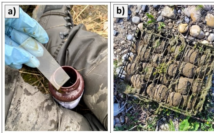
Figure 4.3 Comparison between a) glass slides biofilm and b) rock baskets during method development sampling campaign in June 2021. Larger amounts of biofilms can be obtained through the rock basket method.
