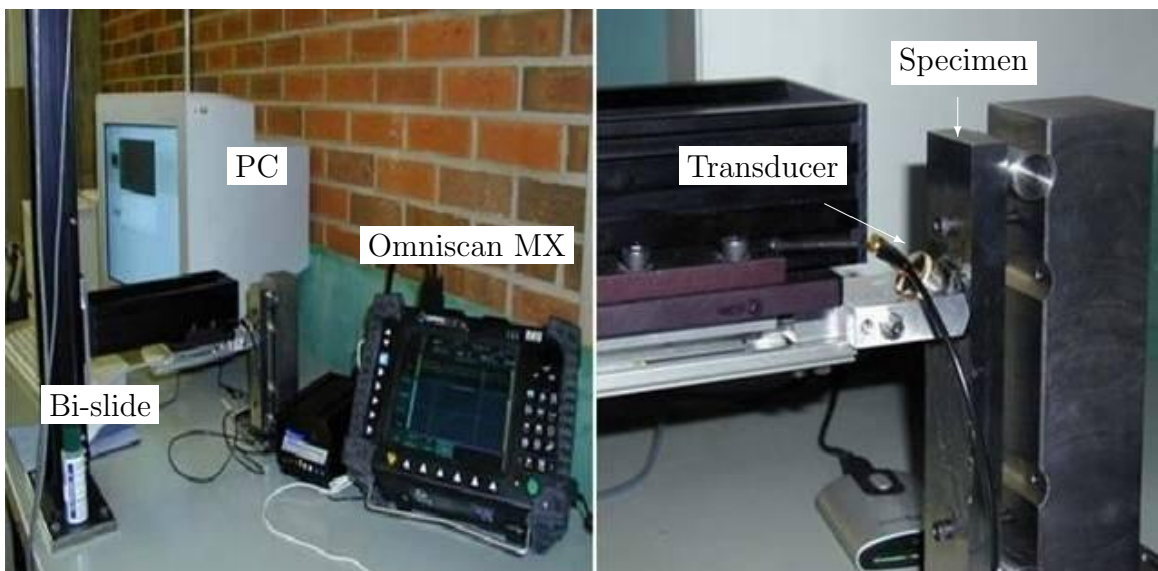
Figure 7.2: Ultrasonic pulse-echo testing using Bi-slide [1]
