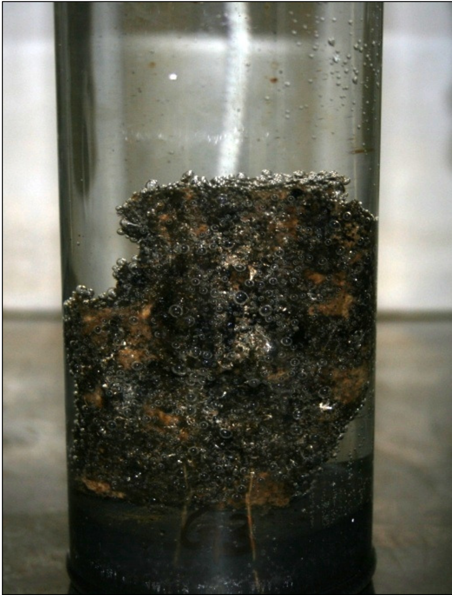
Figure 3-9: Bubbling occurs when sample G4 (the shape is not cylindrical but amorphous) is at the start of Phase-III.
