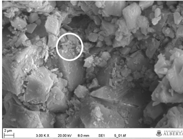
Figure 5-30: SEM image of sample 2 (beated rock) at 3000x.
