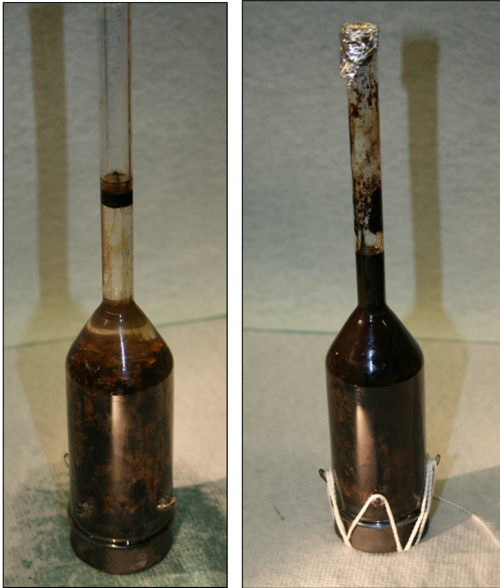
Figure 3-6: Samples G1 in hot water. (a) starting Phase-III, (b) after one week in Phase-III (out of oven).
