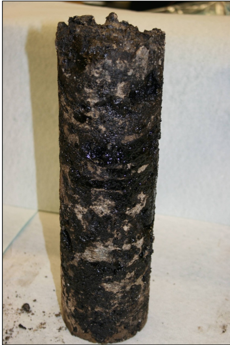
Figure 3-1: Original carbonate core (diameter is ~10 cm).
