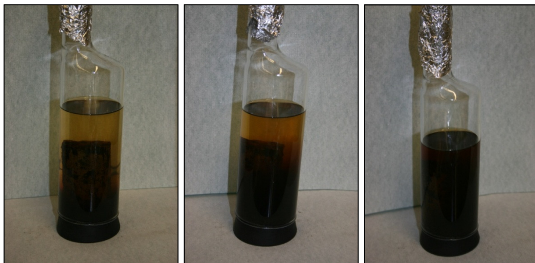
Figure 3-4: Samples G1 in solvent in Phase-II. (a) t=1 min, (b) t=30 min, (c) t=60 min.
