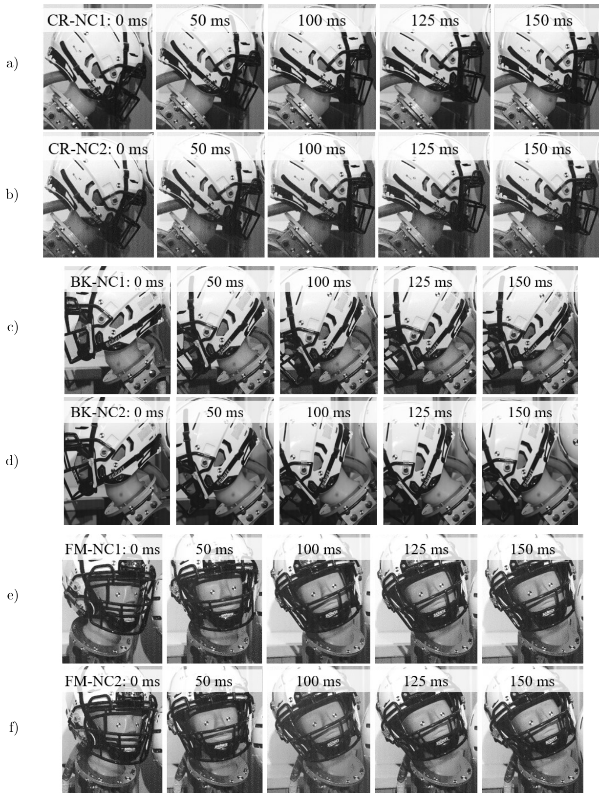
Figure 4.1: Example impact images of PII neck response from low-speed cases: a) CR-NC1, b) CR-NC2, c) BK-NC1, d) BK-NC2, e) FM-NC1, and f) FM-NC2
