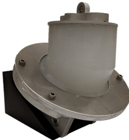
Figure 3.3: Final design form of PII neck with an external silicone casing.
