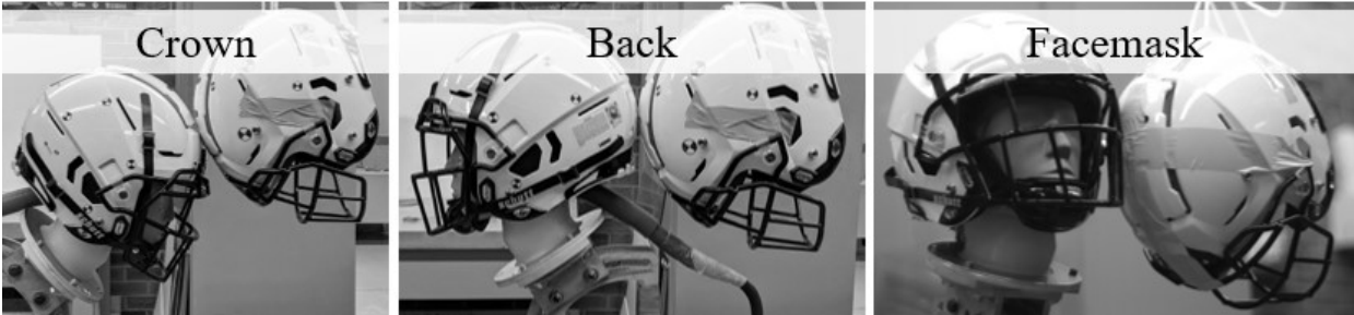
Figure 3.11: Impact location definitions for the crown, back, and oblique facemask.
