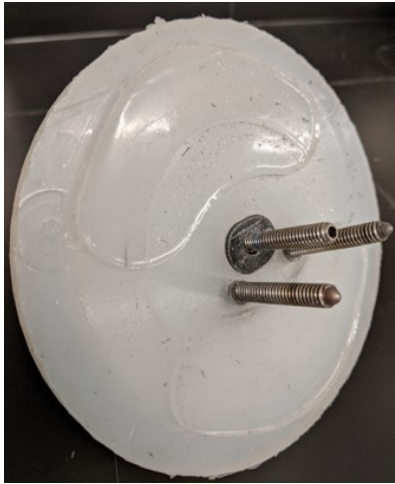
Figure 4.13: No observed damage after impact experiments on the PII neck base.
