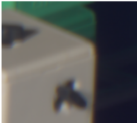
Figure 4.2: A portion of the scene04 image from the KAIST hyperspectral image dataset [19], showing colour fringes from spectral dispersion or other imaging artifacts. Images in this dataset were captured using a monochromatic camera equipped with an apochromatic lens and a liquid crystal tunable filter. The RGB image shown was provided with the dataset.
