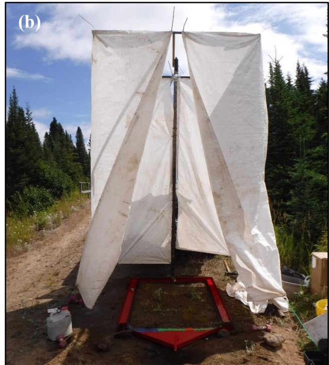
Figure 2.4. Freestanding rainfall simulator used in 2018 (a) and hitch-mounted rainfall simulator used in 2019 (b) with plot frame and collection pan; windbreak is shown in (b).
