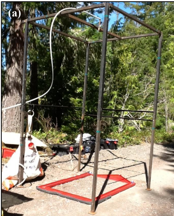
Figure 2.4. Freestanding rainfall simulator used in 2018 (a) and hitch-mounted rainfall simulator used in 2019 (b) with plot frame and collection pan; windbreak is shown in (b).
