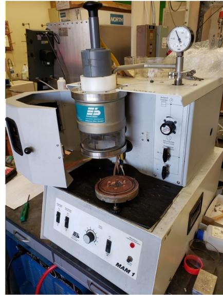
**Figure 1-1.** Solid state synthesis methods: (a) standard resistance furnace and (b) arc melter.
