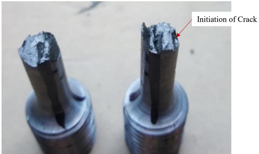
Figure 5-7 Surface of tensile sample showing initiation of cracks along the oxide layers and the brittle fracture of the sample.
