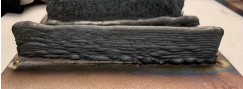
Figure D-2: Wall showing partial adhesion to substrate.
