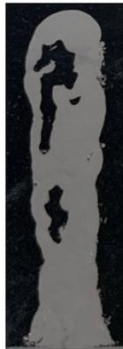
Figure C -1: A cross-section from one of the walls showing cavity.
