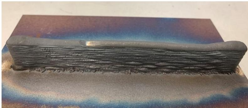
Figure D-1: Wall showing full adhesion to substrate.
