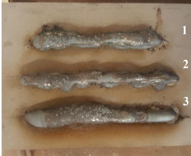
Figure 4-2 Image of the first printed stringer beads.
