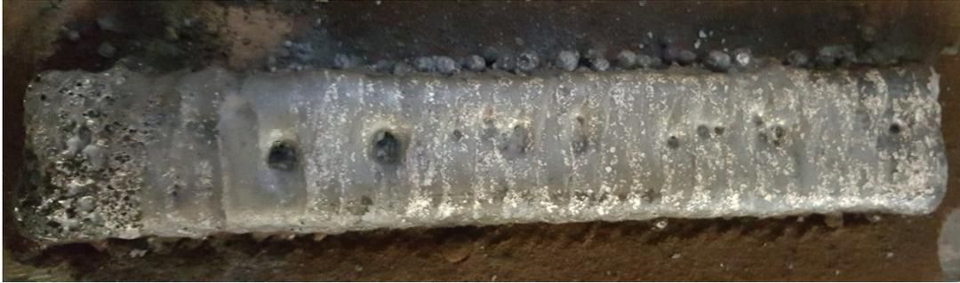
*Figure 4-6 Image of the 10-step weave overlay using nitrogen gas.*
