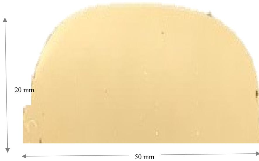
Figure 5-13 Cross section of deposit using powder B showing elimination of both the oxide layers and porosity.
