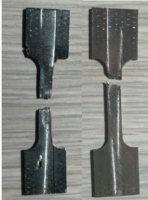
Figure J-1: Tensile fracture mechanisms of three samples from the second DOE. From left to right, sample numbers are square tubes 2-7 CA and 2-7 H900.
