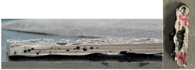
Figure C-4: Images of two cross-sections of the wall built with the minimum peak points.
