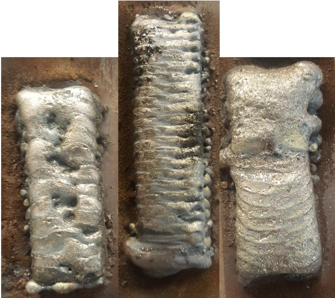
Figure B -1: Samples printed with different process parameters, using nitrogen as a powder gas, showing clear printing surface defects.
