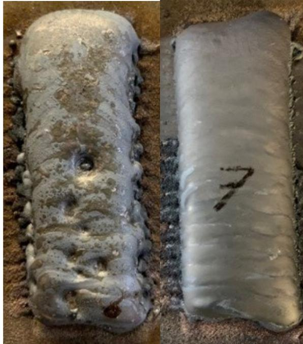
*Figure 5-11 View of the surface of samples fabricated with powder A (left) and powder B (right) using identical process parameters.*
