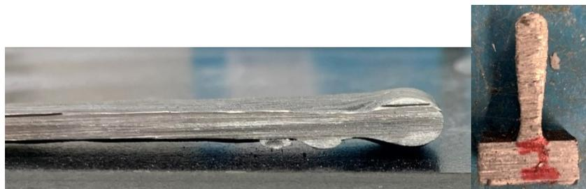
Figure C-3: Imaged of two cross-sections of the wall built with the maximum peak points.
