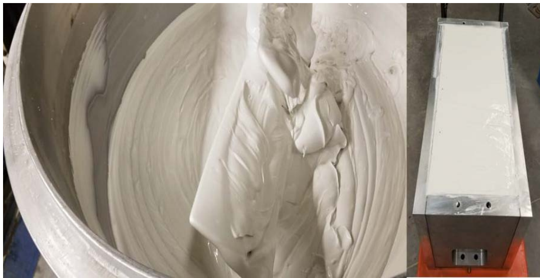
Figure 3-16. Kaolinite slurry: in a vacuum mixer (left) and in the soil container (right)
