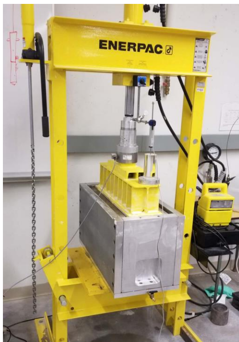
Figure 3-17. Loading frame for kaolinite consolidation
