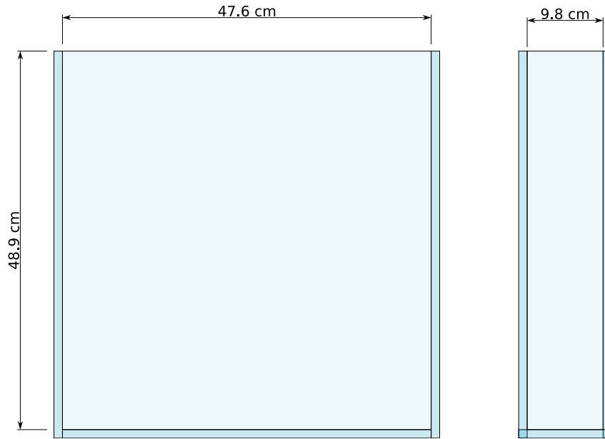
Figure 4.1: Front and side view of tank showing dimensions.
