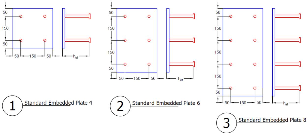
**Figure 3.1 Proposed standard embedded plates (dimensions in mm)**
