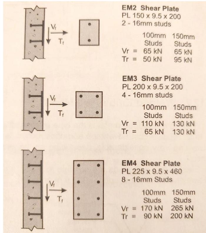
**Figure 2.23 Standard tilt-up panel connectors (CAC 2014)**
