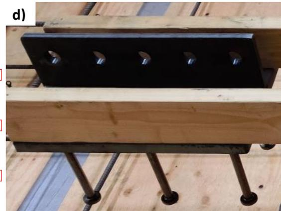
**Figure 4.2 Standardized embedded plates in test program (a) drawing of SEP-04, (b) photo of SEP-04, (c) drawing of SEP-06, (d) photo of SEP-06 suspended in position prior to casting concrete. (All dimensions in mm.)**
