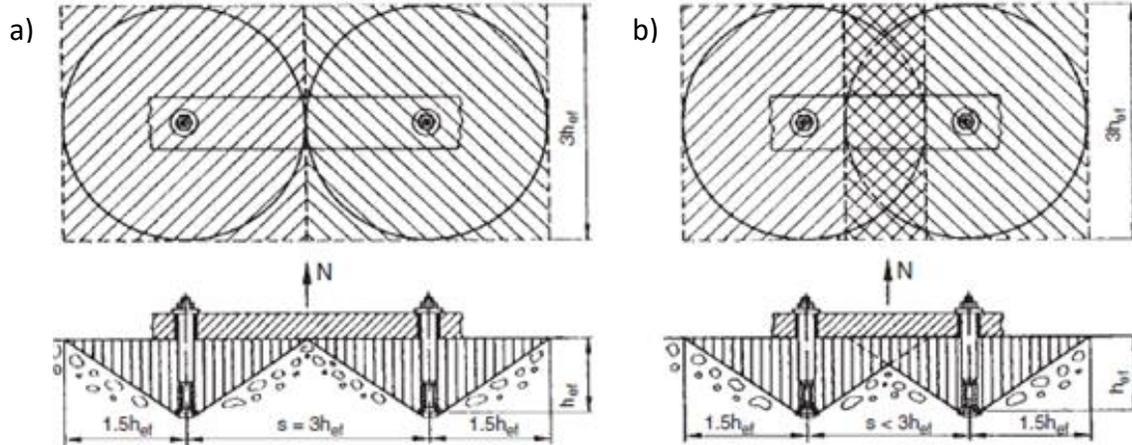
**Figure 2.15 Failure area of an anchor group (Eligehausen et al. 2006): (a) large spacing with no overlapping area; (b) small spacing with overlapping area**
