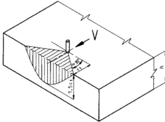
**Figure 2.6 Concrete breakout in shear (Fuchs et al. 1995)**
