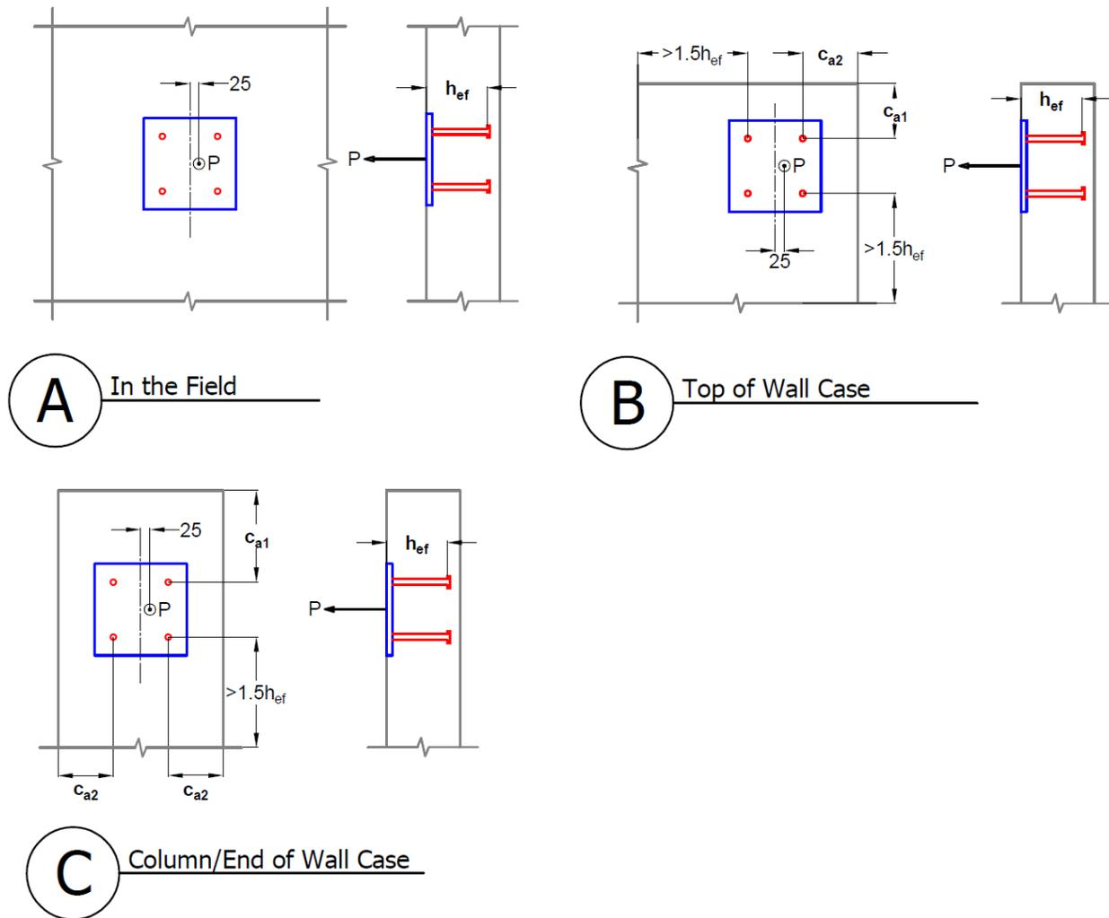
**Figure 3.3 Embedded plate design cases for tensile load**
