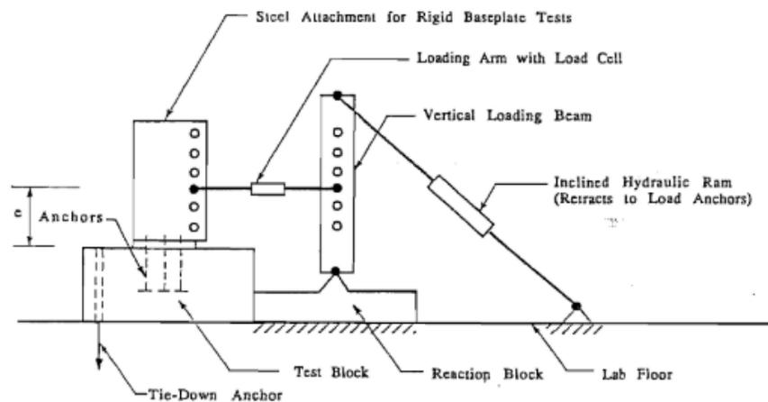
**Figure 2.13 Schematic diagram of test-setup (Cook et al. 1989)**
