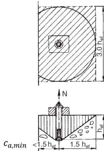
**Figure 2.17 Influence of edge distance on concrete cone failure surface (adapted from Eligehausen et al. 2006)**
