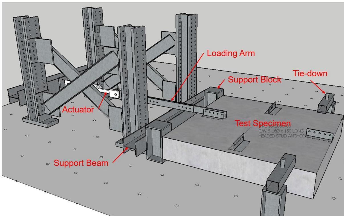
**Figure 4.6 Test setup**
