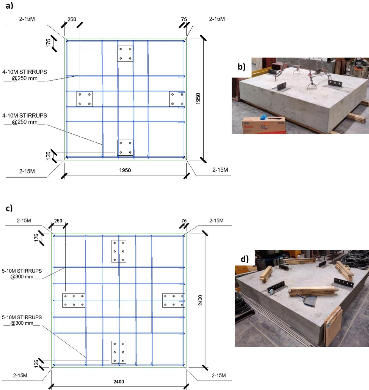
**Figure 4.3 Assemblies used in test program (a) drawing of concrete specimen for SEP4 tests (b) photo of concrete specimen for SEP4 tests (c) drawing of concrete specimen for SEP6 tests (d) photo of concrete specimen for SEP6 tests. (All dimensions in mm.)**
