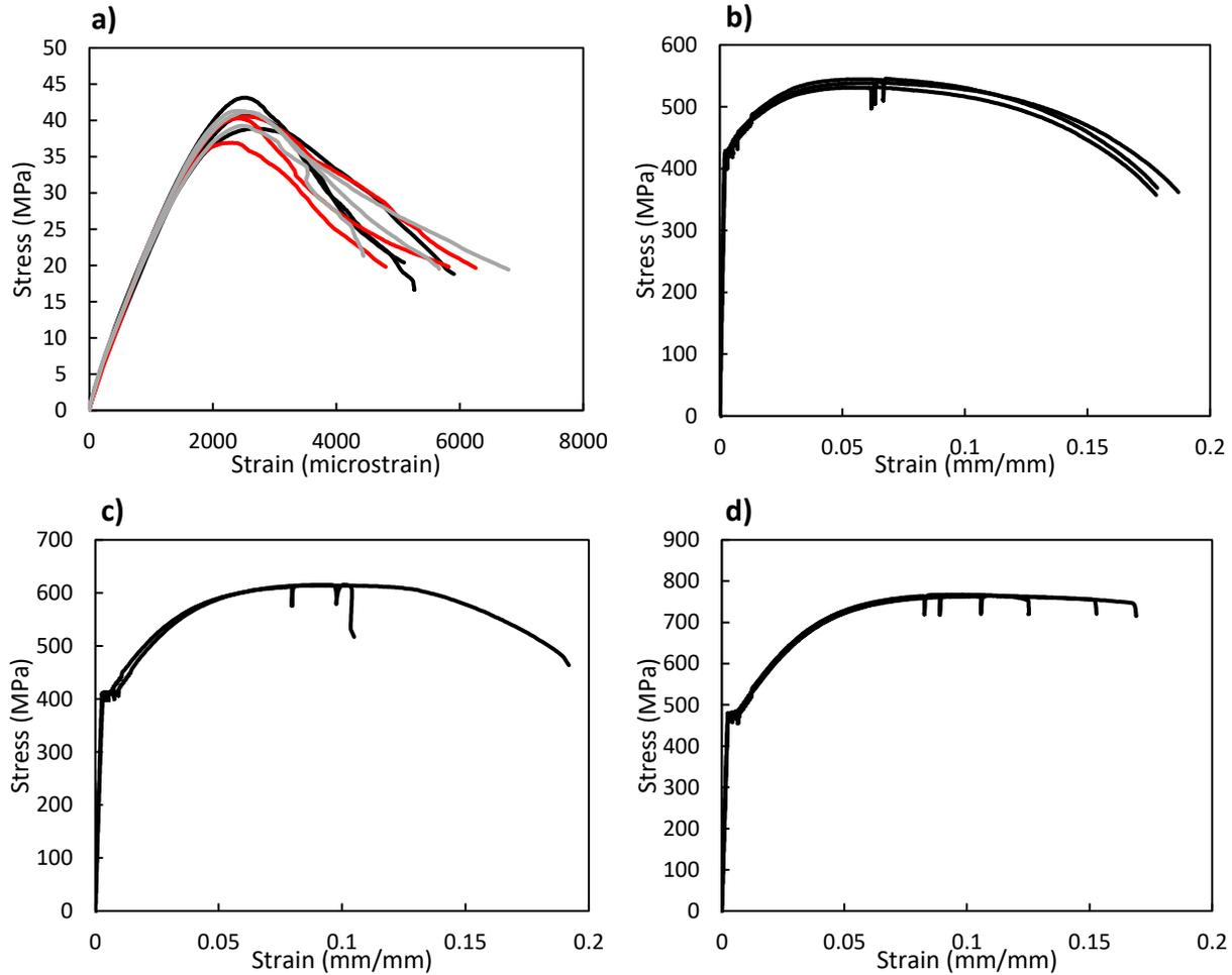
**Figure 4.5 Stress–strain curves of (a) concrete cylinders (black) right before first full-scale test, (red) after 4 full-scale tests, (grey) after all 8 full-scale tests (b) headed studs (c) 10M rebar (d) 15M rebar**
