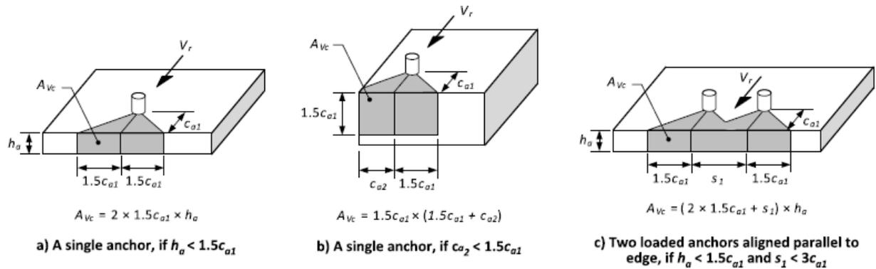
**Figure 2.20 Concrete breakout failure area of single anchor and anchor group in shear (CSA 2019)**
