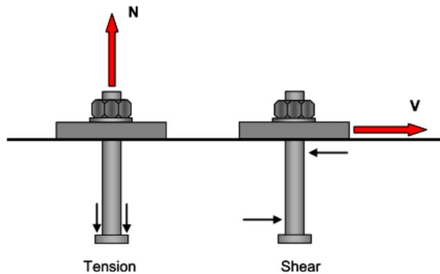
Figure 1.2 Anchor load transfer mechanisms (Grosser 2012)
