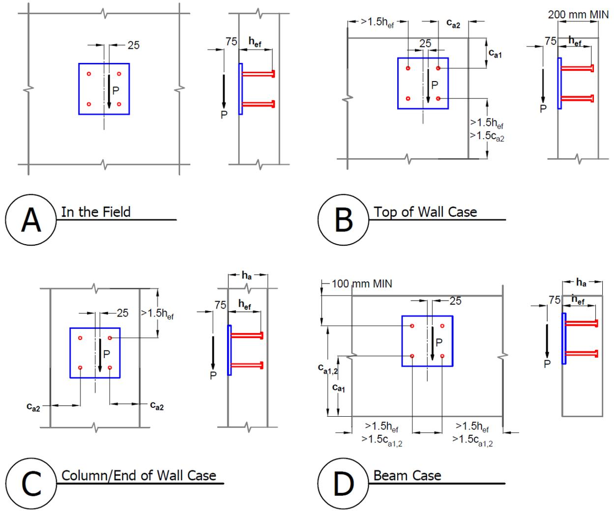
Figure 3.2 Embedded plate design cases for shear load
