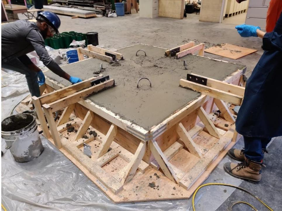
**Figure D.5 Finishing of SEP4 concrete specimen**
