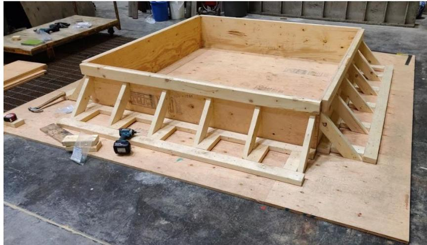
**Figure D.1 Formwork for SEP4 concrete specimen**
