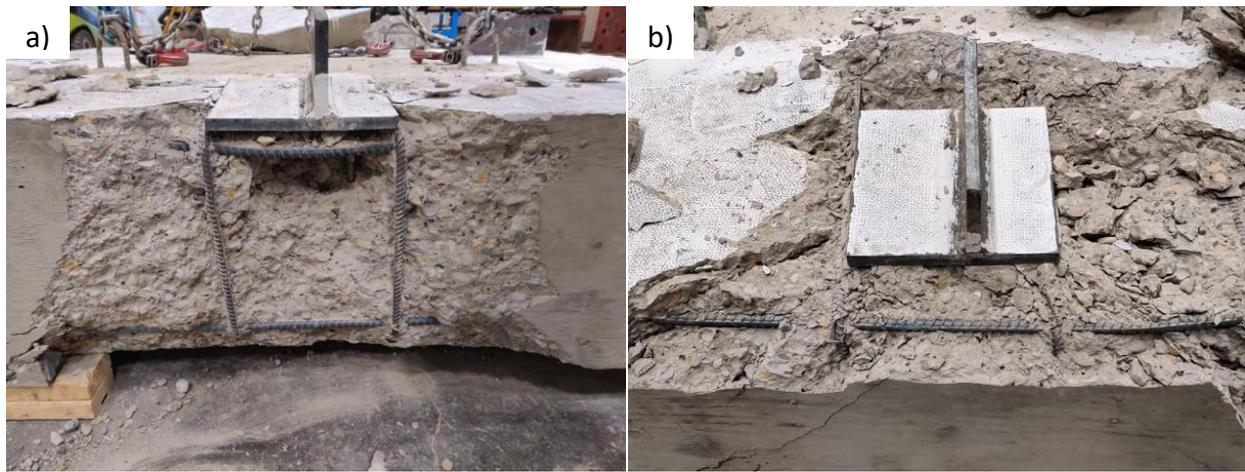
**Figure 4.10 Edge reinforcement after testing of (a) SEP4-150-125 and (b) SEP4-150-175**
