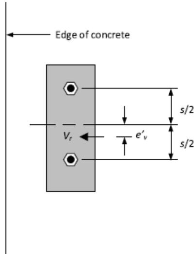
**Figure 2.21 Eccentricity of shear load an anchor group (CSA 2019)**
