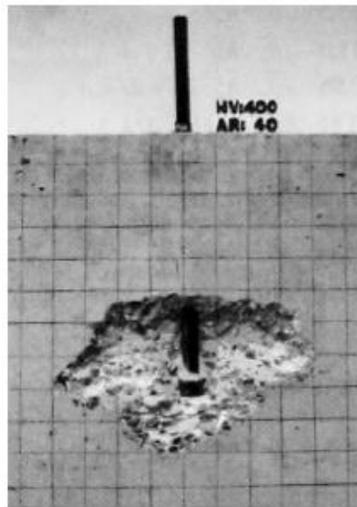
**Figure 2.4 Concrete side-face blowout (Eligehausen et al. 2006)**
