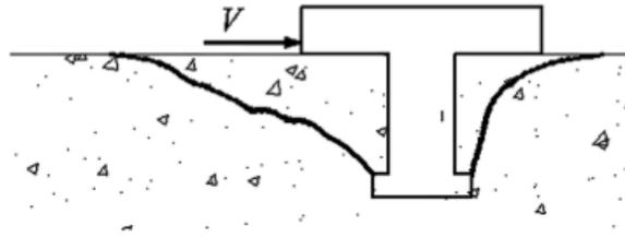
**Figure 2.11 Concrete pryout failure (Jebara et al. 2015)**
