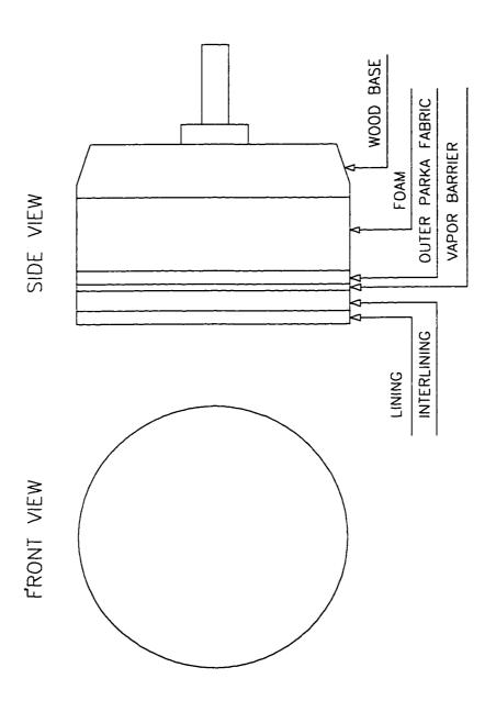
Figure 2. Rubbing materials attached to the rubbing wheel in the order present in the parkas worn in the human-body experiment.
