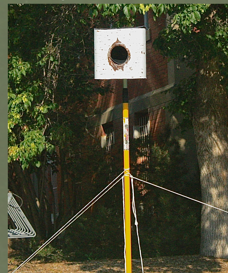
Figure 3: Synthetic cavity on an adjustable pole to determine controls needed for trigonometry to be used.
