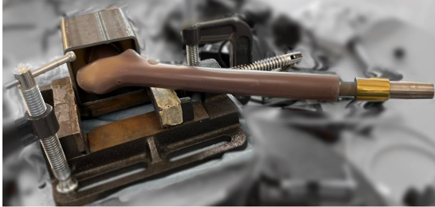
Figure 3-13. The boundary condition was changed from a free end (Figure 3-8) to a cantilever. The femoral head (excluding the neck and the trochanter) is fixed in a resin block to simulate a cantilever boundary condition.
