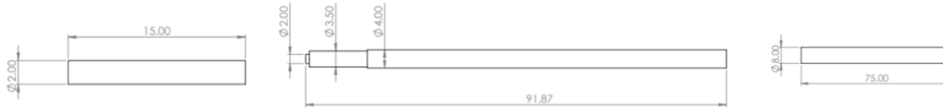
Figure 5-6 Particle (Left), Periotest® (Middle) and the 30g rod (Right) geometries used in the 3D FE simulation. The particle's density is adjusted to end up with 9.4g and 30g. The sketches are not to scale.
