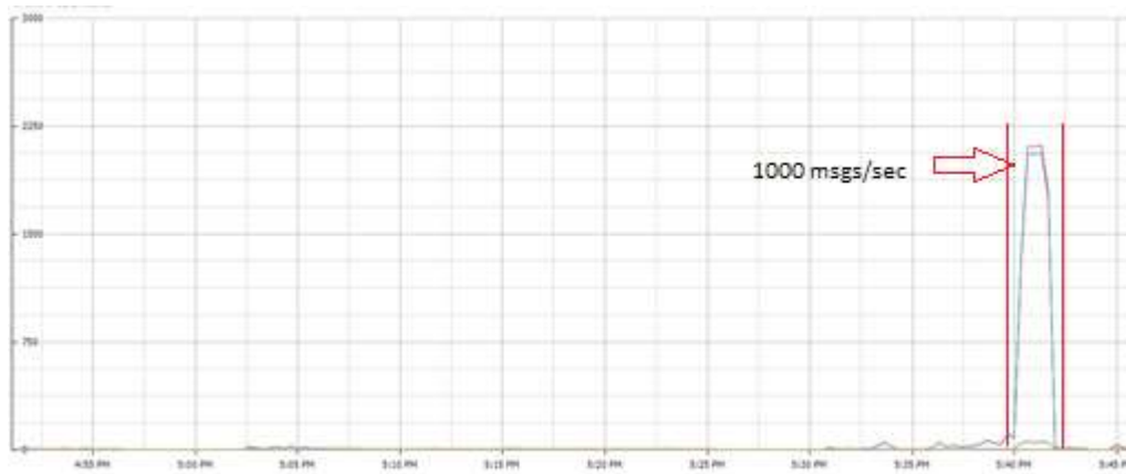
Figure-43. VMware Network performance monitor. Using TLS
