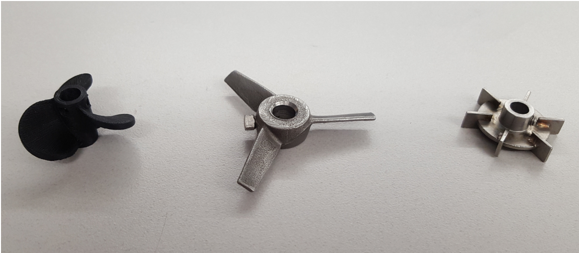
Figure 2.9: Marine (left), Lightnin A310 hydrofoil (middle), and Rushton (right) impellers.
