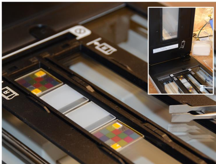
Figure 3-7 Consumer flatbed film scanner (Canon 9000F) used to image GLAD UTLC media before and after development. A light source built into the scanner lid transmits light through the translucent plates into the detector below (inset).
