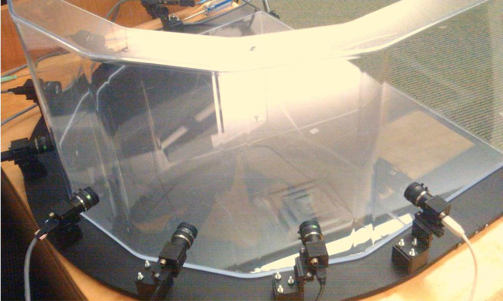
**Figure 4.2:** Our tank array has a different side for each camera. Since cameras do not share the same refractive interface, we need a model which takes into account that each camera is behind a different refractive interface.
