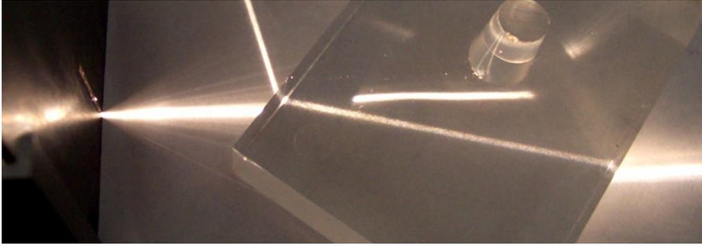
**Figure 3.5:** Illustrating refraction in a block of Perspex. (Source: <http://en.wikipedia.org/wiki/File:Refraction.jpg>)
