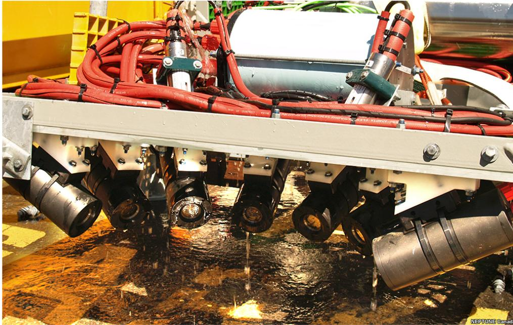
**Figure 1.1:** The 8-camera array deployed at the Folger Pass station of the NEPTUNE project. This camera array will be used to observe and reconstruct organisms in 3D. (Source: [NEPTUNE Canada](#))
