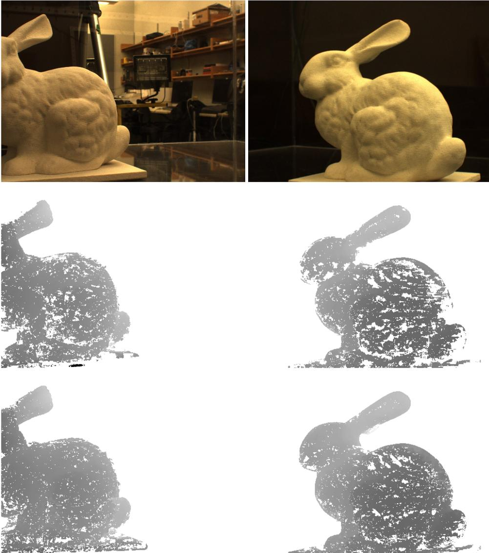
**Figure 2.13:** Example results from our implementation of the method of Campbell et al. [7]. Two different views of the Stanford bunny model (top row) and the resulting depth maps produced when using three (middle row) and eight views (bottom row). More views provide better peaks, which reduces the number of pixels being labelled as “unknown” (white pixels).
