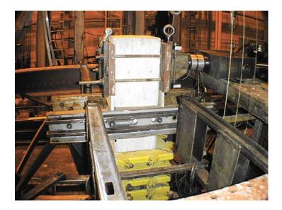
Figure 4-14(a): Photograph showing the attachment of horizontal loading assembly to the column specimen
