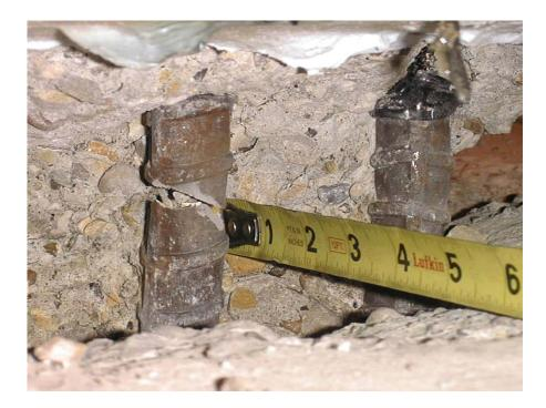
Figure 4-25: A close-up of ruptured longitudinal bars of specimen CL6 at the end of test
