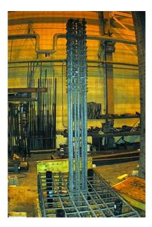
Figure 4-3: Photograph showing the reinforcement of a typical collared column with no splicing in the longitudinal bars of the column
