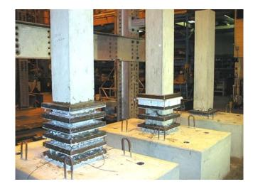
Figure 1-8: Three of the nine phase 2 columns at different stages of collar installation
