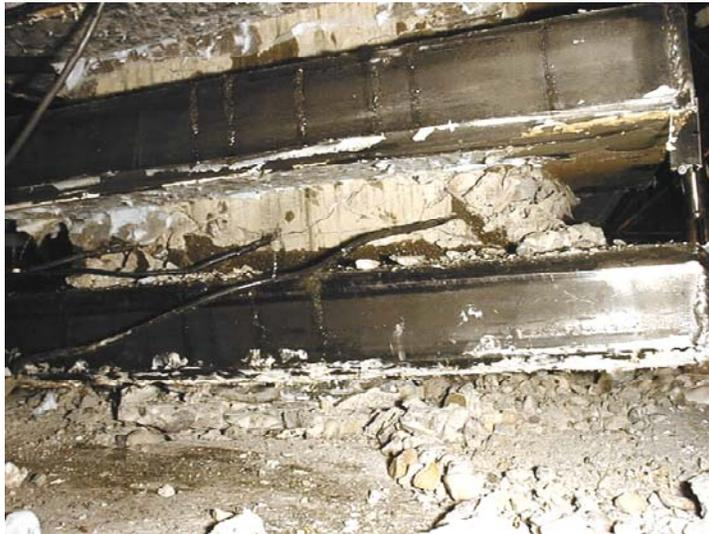
(d) a view of damage in gaps 1 and 2 at test end
