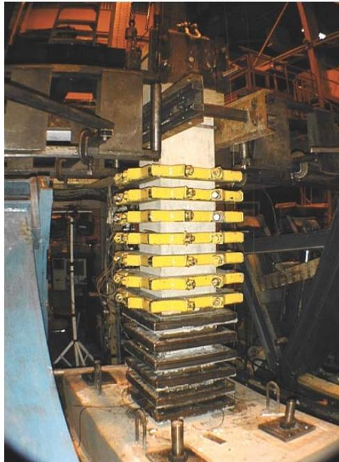
Figure 1-9: A typical phase 2 column in the test set-up.
