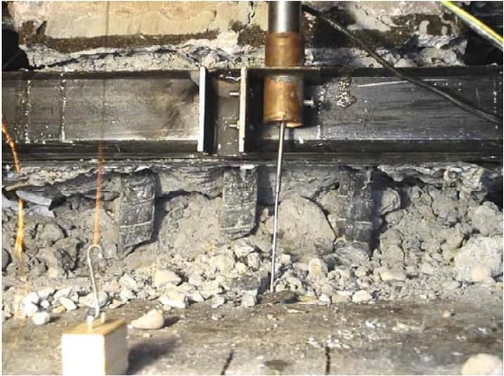
(c) a close-up of lower portion (ruptured bars visible)
