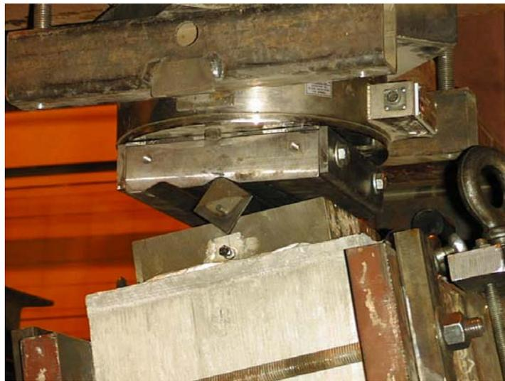
Figure 4-14(b): Photograph showing the knife edge support and flat load cell for measuring vertical loads
