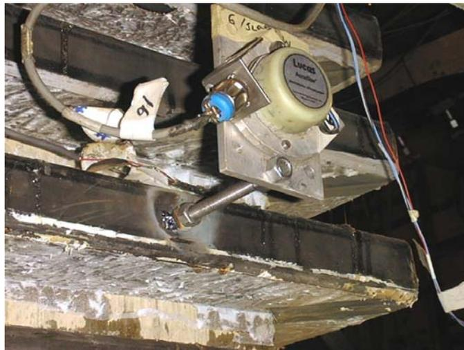
Figure 4-16: Photograph showing rotation meter for measuring the rotation of collars
