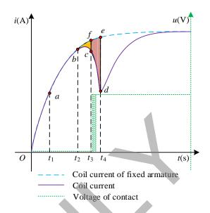
Fig. 7. Coil current and contact potential of the contactor.
