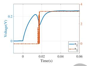
Fig. 12. Coil current  $u_2$ , contact potential  $u_3$ .
