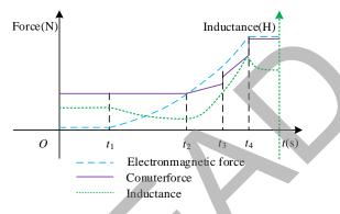
Fig. 8. Electromagnetic force, counterforce and inductance in the movement.
