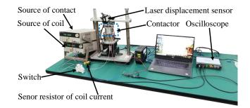
Fig. 17. Test platform for model verification.
