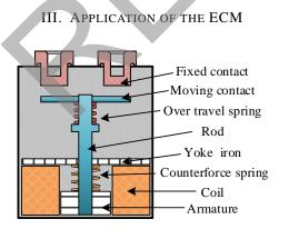
Fig. 9. Internal structure of the contactor.
