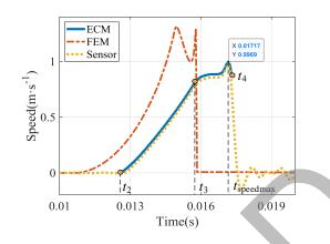
Fig. 18. Comparison of speed in ECM, FEM, and sensor.
