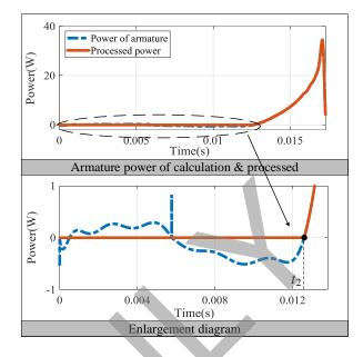
Fig. 16. Armature power in the transient process.
