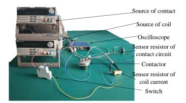
Fig. 10. Coil current sampling circuit experiment.
