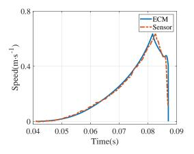
Fig. 22. Comparison of speed in ECM and sensor for 750V/630A contactors.
