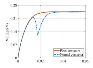
Fig. 5. Coil current (sampling voltage of  $u_2$  in Fig. 11) of fixed armature and normal contactor.
