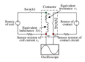
Fig. 11. Coil current sampling equivalent circuit.
