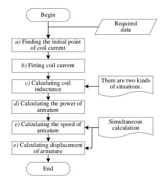
Fig. 14. Flow chart for calculating ETCs.
