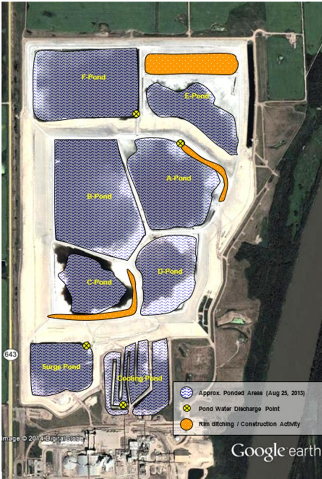
Figure 2.1. Map of active process ponds on the phosphogypsum stack at the Agrium Redwater Operation Facility.
