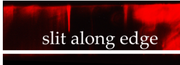
Figure 2.4: Fluorescence image of the fiber showing the hypothetical spectrometer slit alignment.
