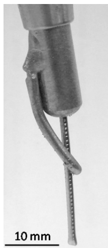
Figure A.4 "Bend-back" type contact tip used in this study.
