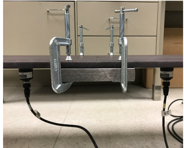
(b) DC2: Added mass at mid-span
