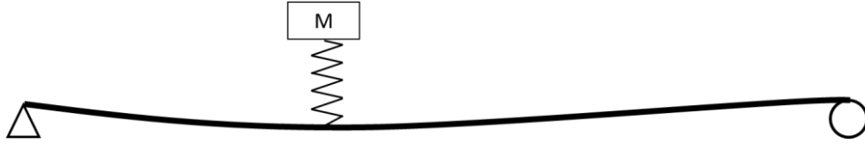
Figure 3.6 - Spring mass vehicle bridge interaction model (adapted from [44])
