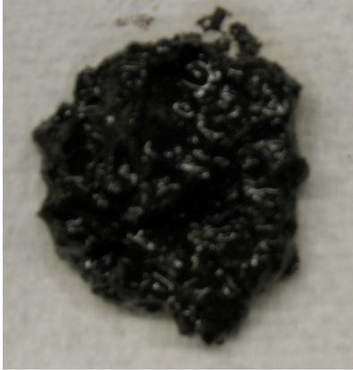
**Figure 31: Untreated drill cuttings containing D822 base oil**
