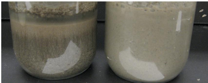
**Figure 41: Untreated 1:1 slurries containing just drill cuttings (left), and drill cuttings previously mixed with additive (right), after about 2 minutes of settling**
