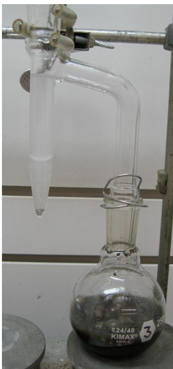
**Figure 16: Dean-Stark extraction set-up. The toluene and drill cuttings are placed in the flask (bottom right), and the water is collected in the Dean-Stark trap (upper left)**
