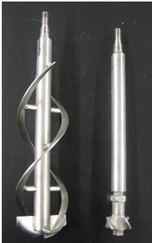
**Figure 14: Helical mixing impeller (left) that permits CO<sub>2</sub> inlet just above blade, approximately 2.5 inches below the top of the vessel, and paddle impeller (right) that permits CO<sub>2</sub> inlet at bottom of vessel**
