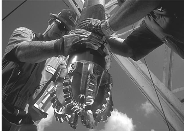
**Figure 3: Drill bit and drill string (taken with permission from [3])**
