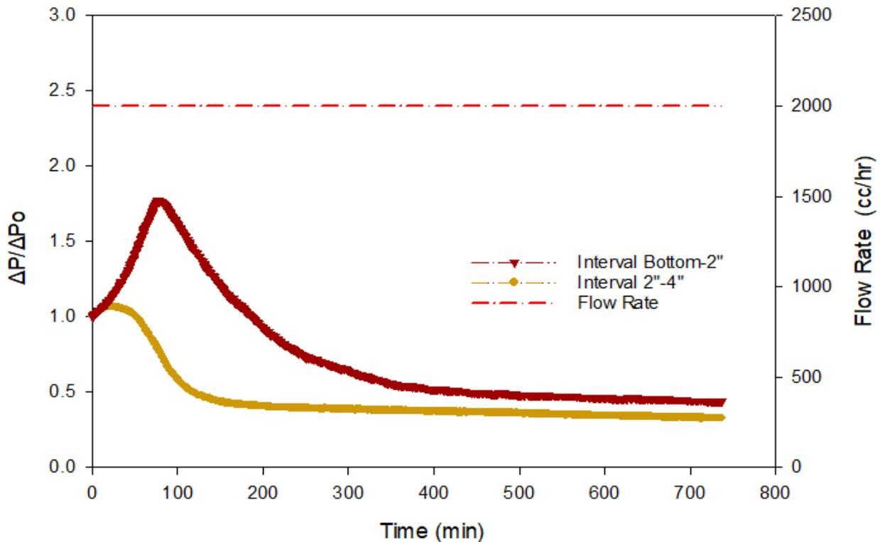
**Figure 4.4:** Dimensionless pressure drop variations for the first flow stage using a wire mesh screen.
