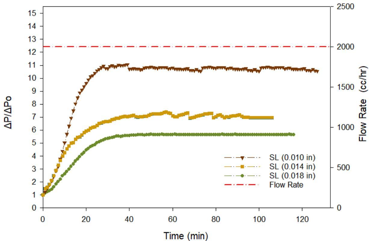
**Figure 4.6:** Near-screen dimensionless pressure drop for different SL screens, injecting 400 ppm brine.
