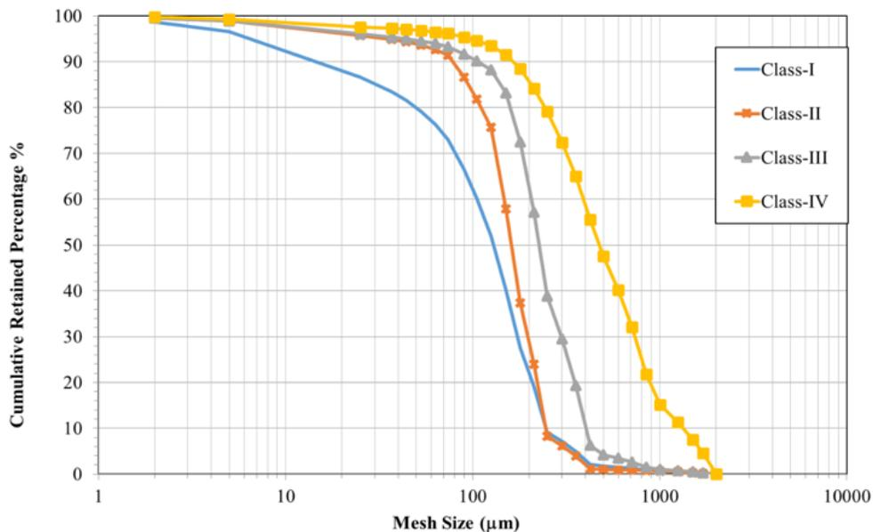
**Figure 2. 3:** PSD of the representative classes of oil sand in McMurray Formation [4].
