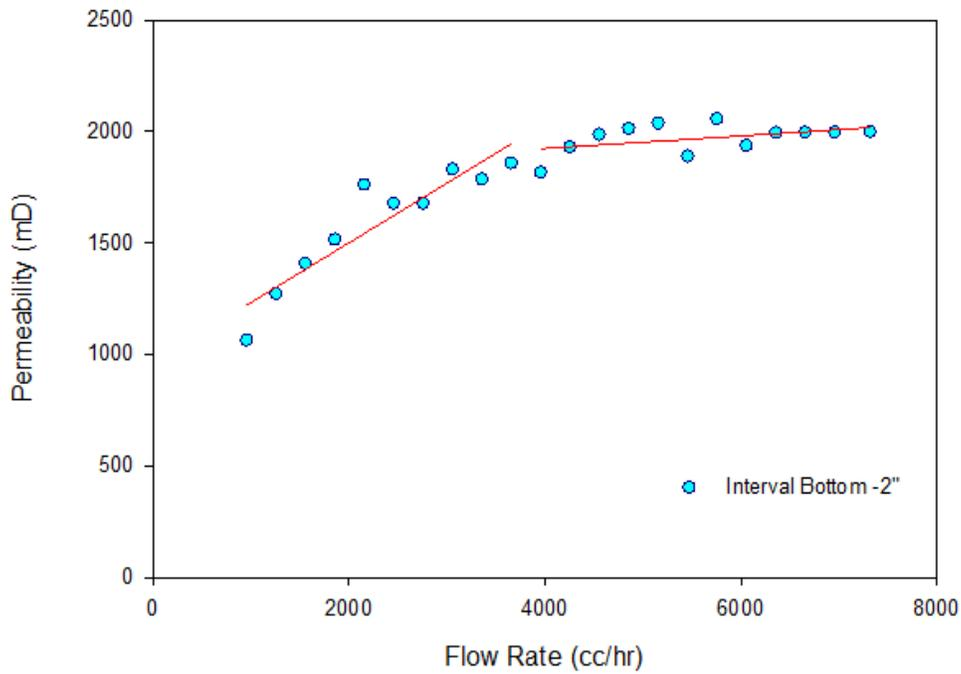
**Figure 3. 22:** Permeability variation with increasing flow rate -Bottom interval (0-2") of a fines-free sand pack.
