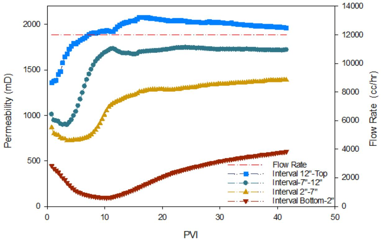
Figure 3. 11: Instant permeability variations at four intervals of the sand pack-Test No. 2.
