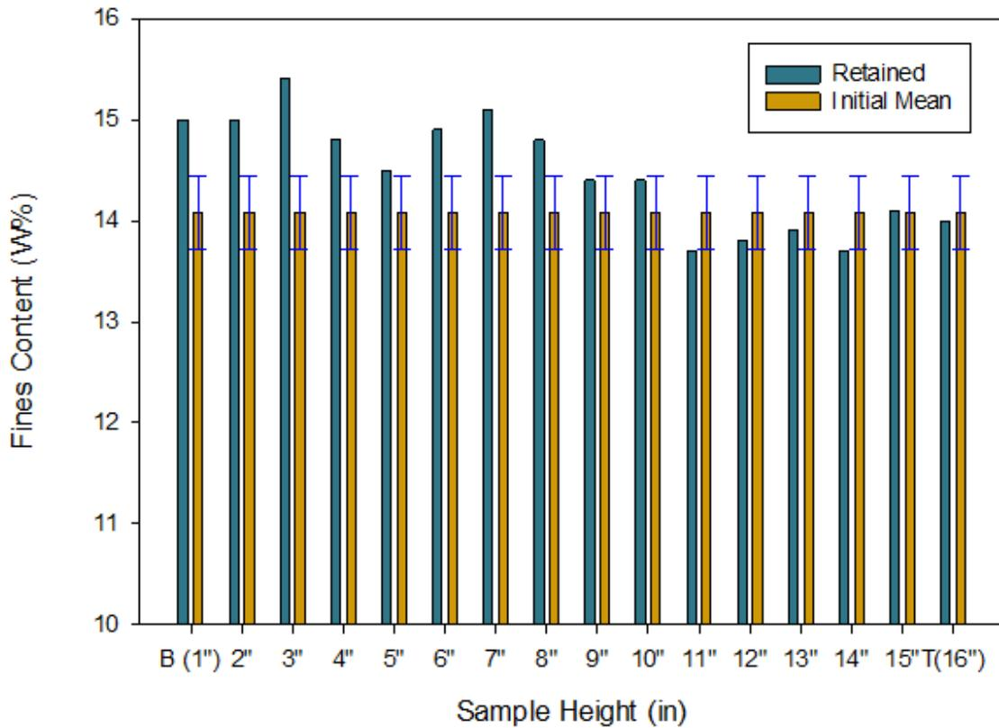
Figure 3. 9: Initial and retained fines content profile -Test No. 1.
