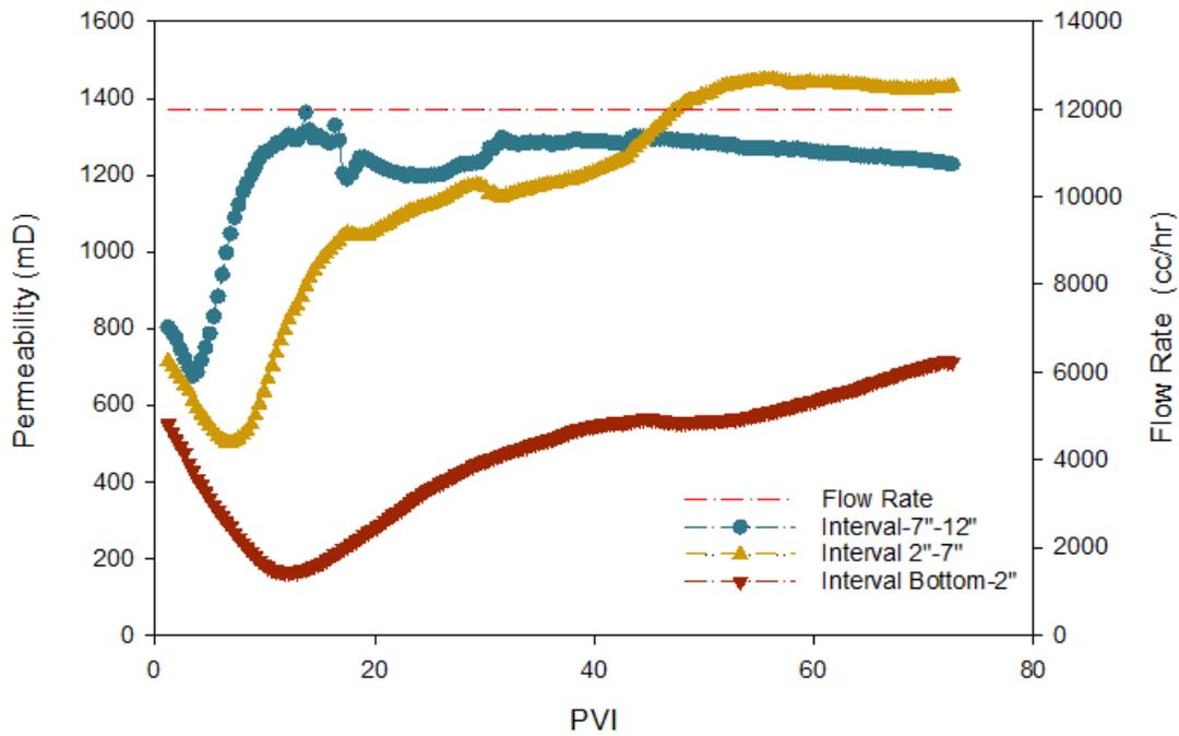
**Figure 3. 7:** Instant permeability variations at three intervals of the sand pack-Test No. 1.
