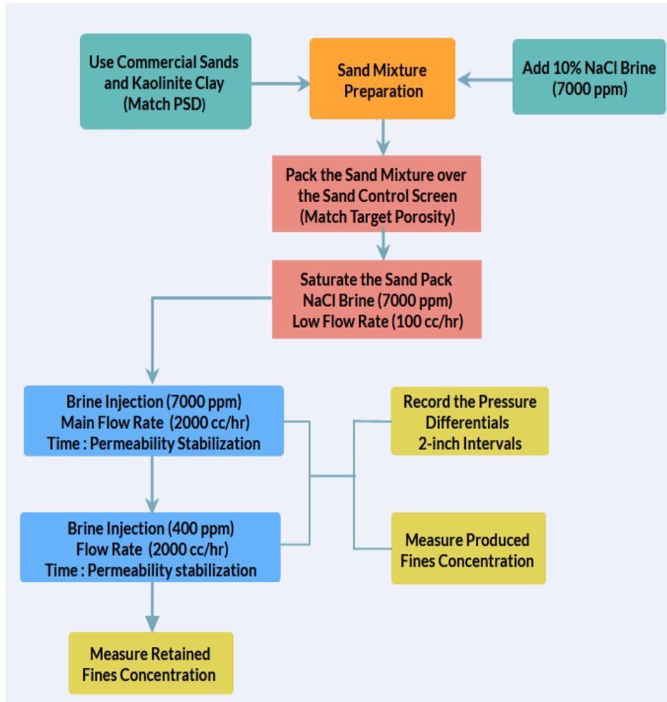
**Figure 4.3:** The testing procedure flowchart.
