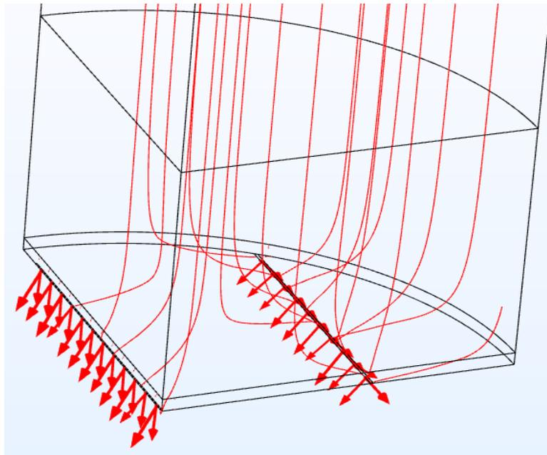
Figure 4A. 2: Flow streamlines, converging toward slot openings.
