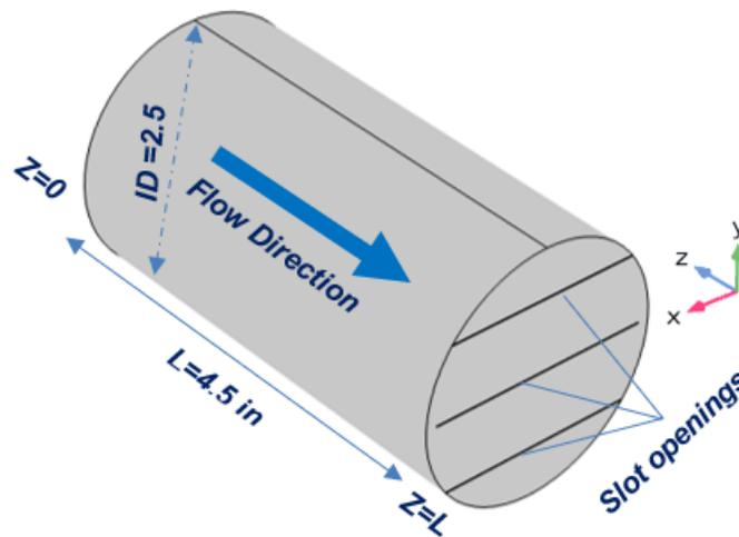
**Figure 4.12:** The schematic of the numerical model geometry.
