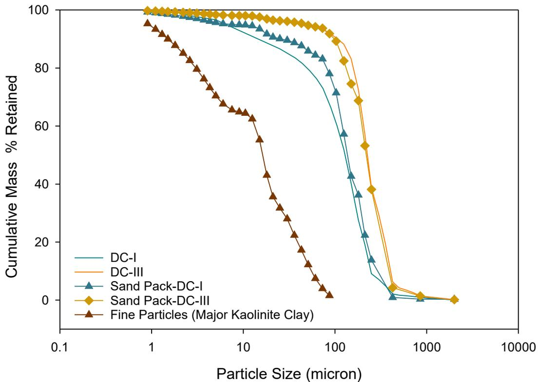
**Figure 3. 3:** Particle size distribution of formation sands, sand packs, and fine particles.
