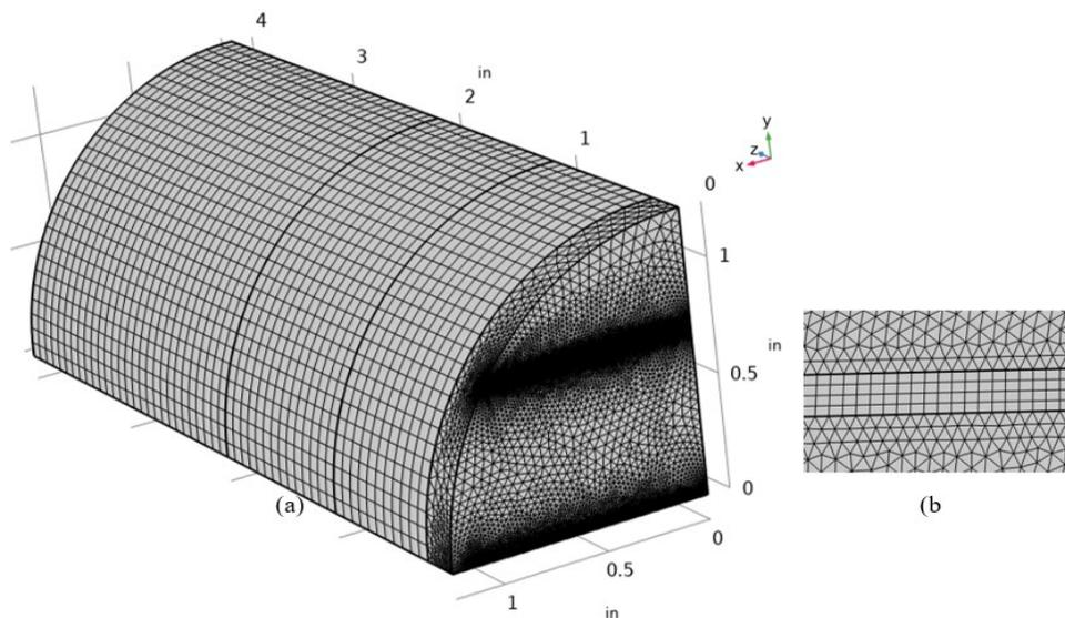
**Figure 4.13:** Illustration of (a) the mesh used and (b) mesh elements across one screen slot.
