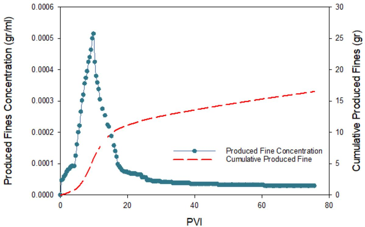
Figure 3. 8: Produced fines concentration versus injected pore volume -Test No. 1.
