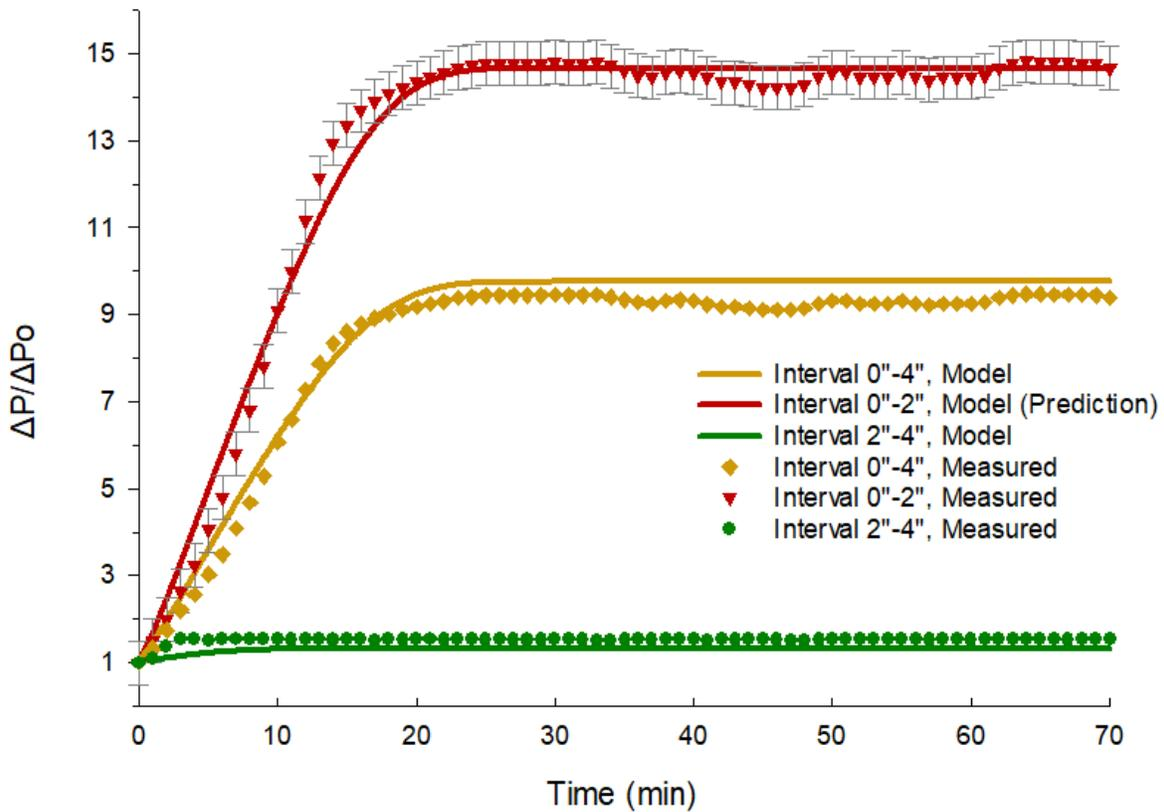
Figure 4. 19: The matched and predicted dimensionless pressure drops with error bars for the test using SL 0.010" and injecting 200 ppm brine.
