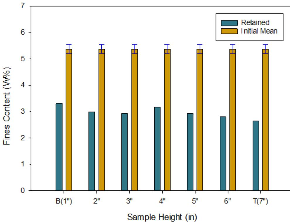
**Figure 3. 19:** Initial and retained fines content profile -Test No. 5.
