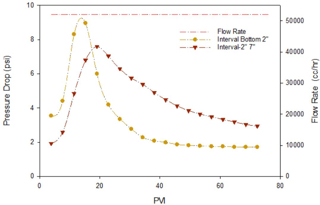
**Figure 3. 20:** Instant pressure drop variations at two intervals of the sand pack-Test No. 6.
