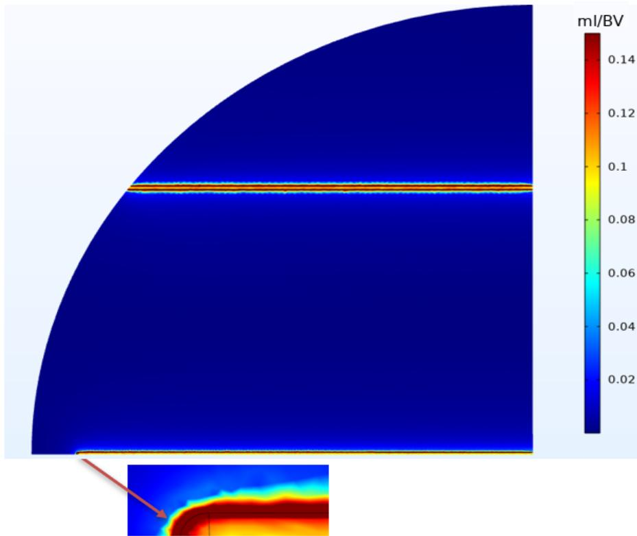
Figure 4A. 5: Retained fines concentration map near the slots after fines migration process, SL 0.010", 400 ppm brine flow, top view.
