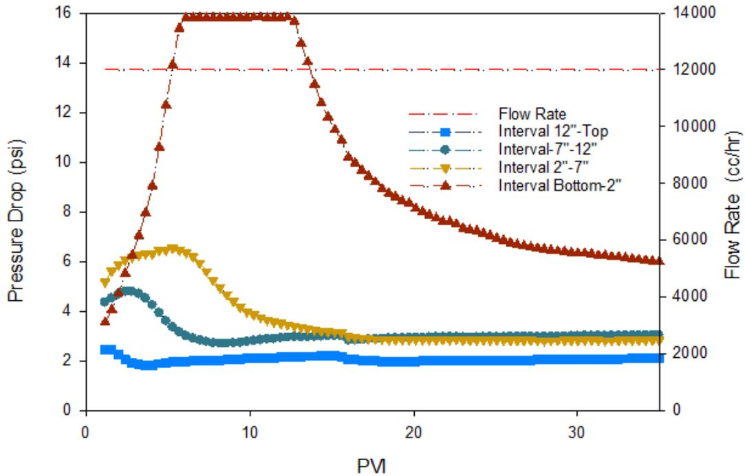
**Figure 3.14:** Instant pressure drop variations at four intervals of the sand pack-Test No. 3.
