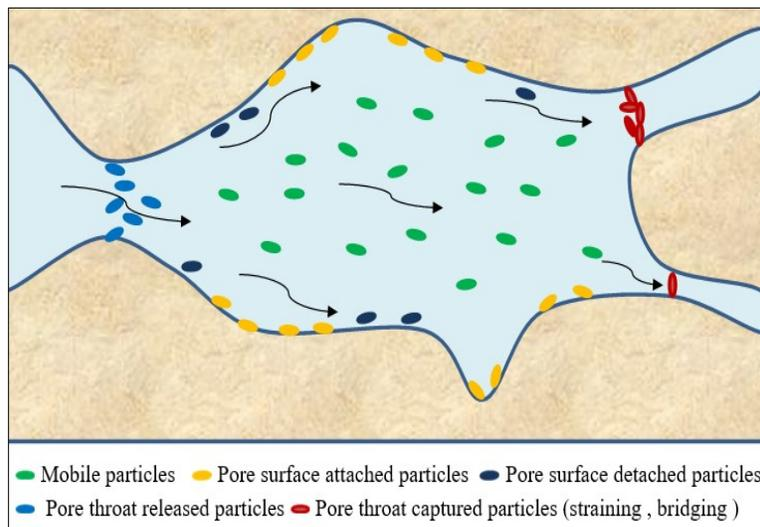
**Figure 3. 1:** Schematic of fine particles release, migrate and capture mechanisms in a pore space [17].
