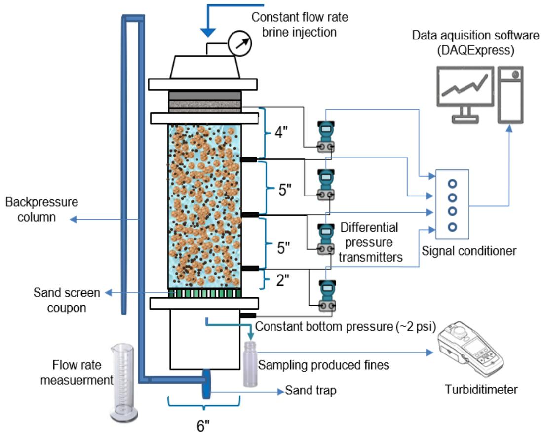
**Figure 3. 2:** Schematic of different components of the sand retention testing set-up.
