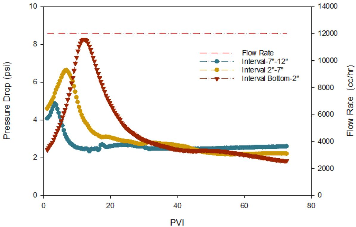
**Figure 3. 6:** Instant pressure drop variations at three intervals of the sand pack-Test No. 1.
