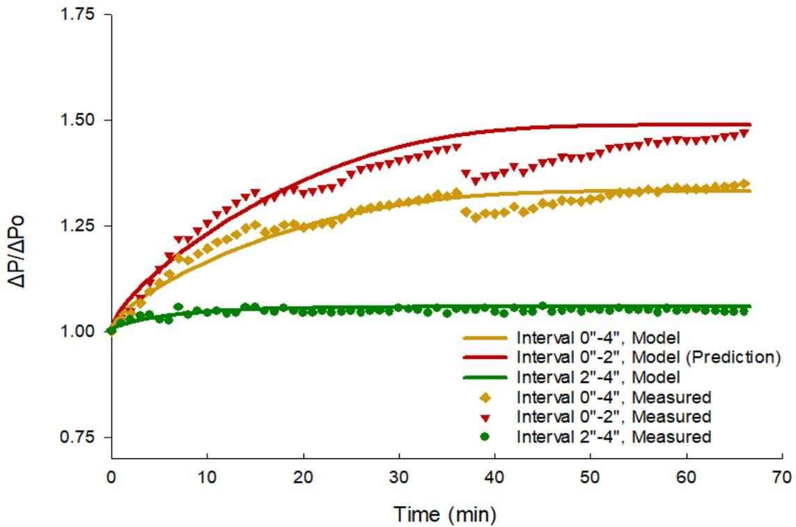
Figure 4. 18: The matched and predicted dimensionless pressure drops for the test using SL 0.010" and injecting 800 ppm brine.
