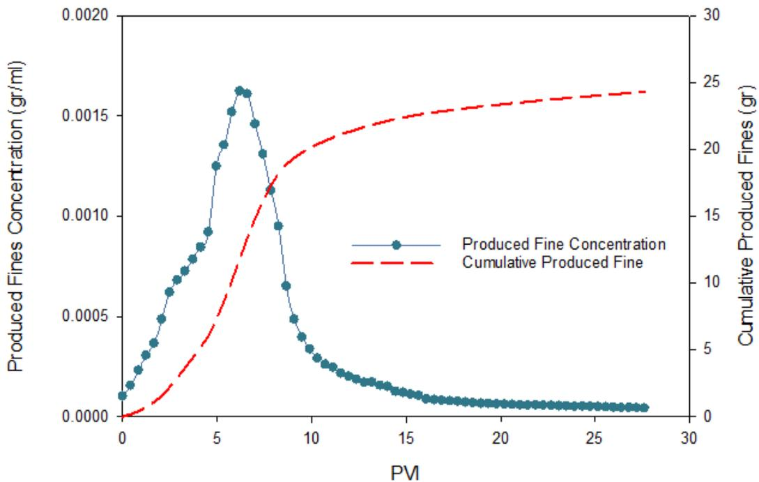
**Figure 3.15:** Produced fines concentration versus injected pore volume -Test No. 3.
