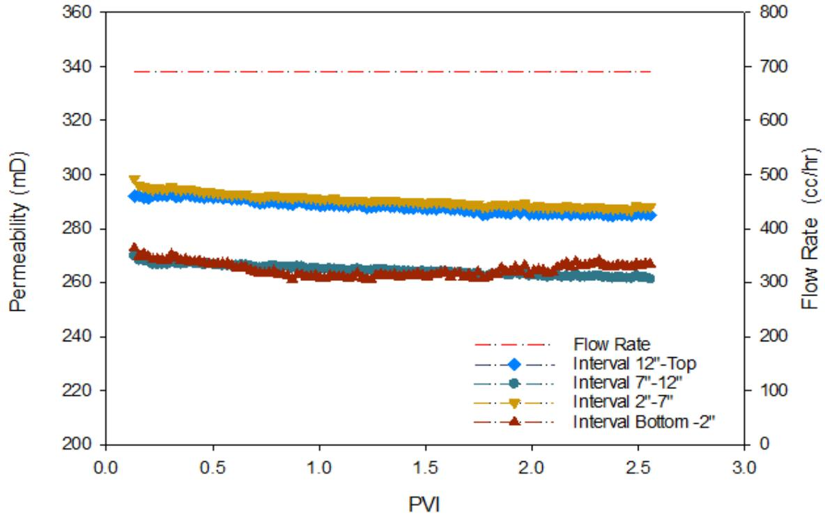
**Figure 3. 5:** The initial permeability of four intervals of the sand pack- Test No. 1.
