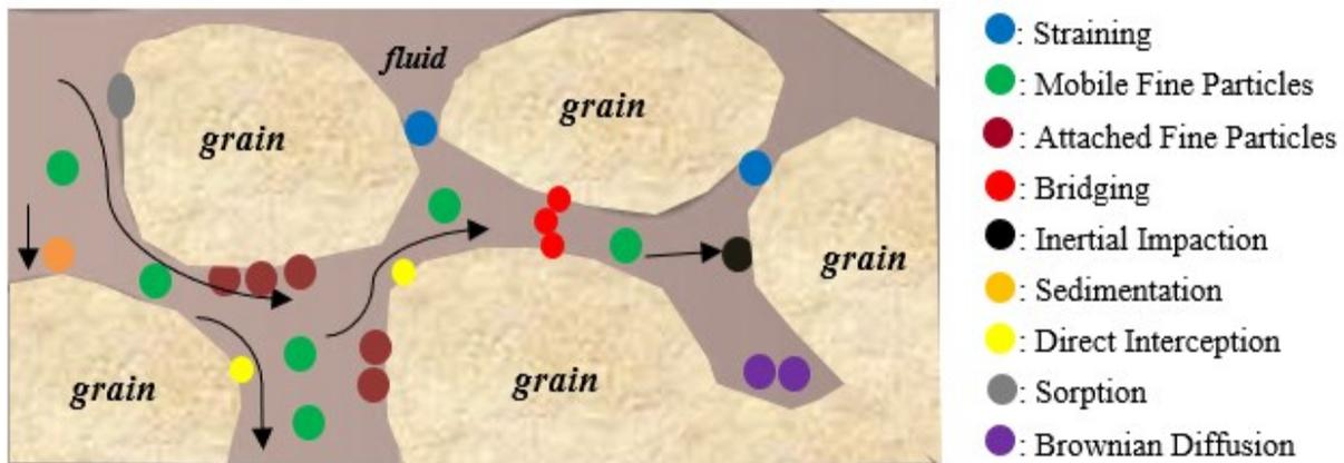
**Figure 2. 9:** Different mechanisms of particle retention in porous media.
