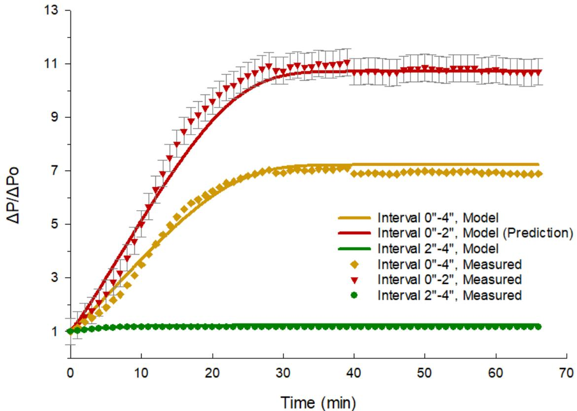
**Figure 4. 15:** The matched and predicted dimensionless pressure drops with error bars for the test using SL 0.010" and injecting 400 ppm brine.
