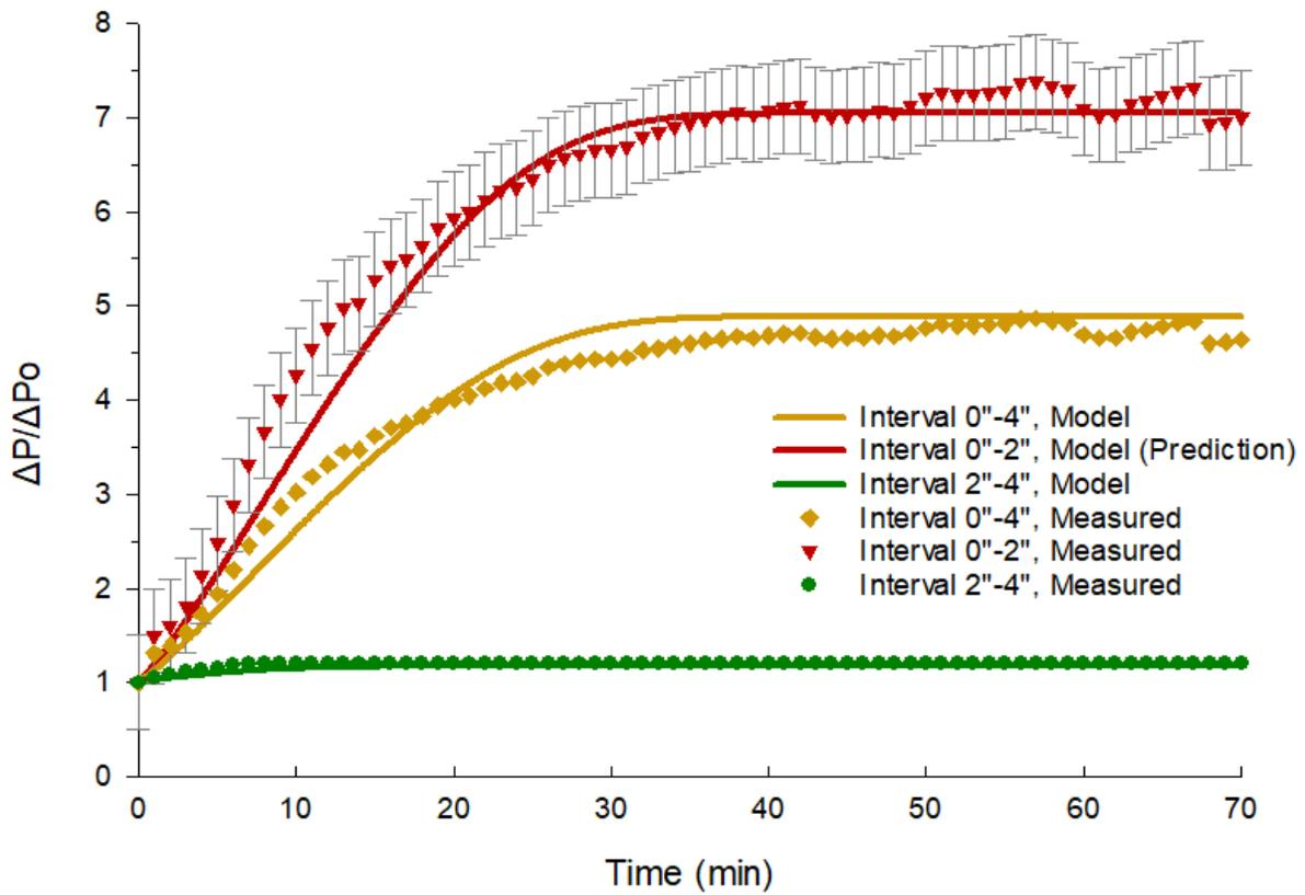
Figure 4. 16: The matched and predicted dimensionless pressure drops with error bars for the test using SL 0.014" and injecting 400 ppm brine.
