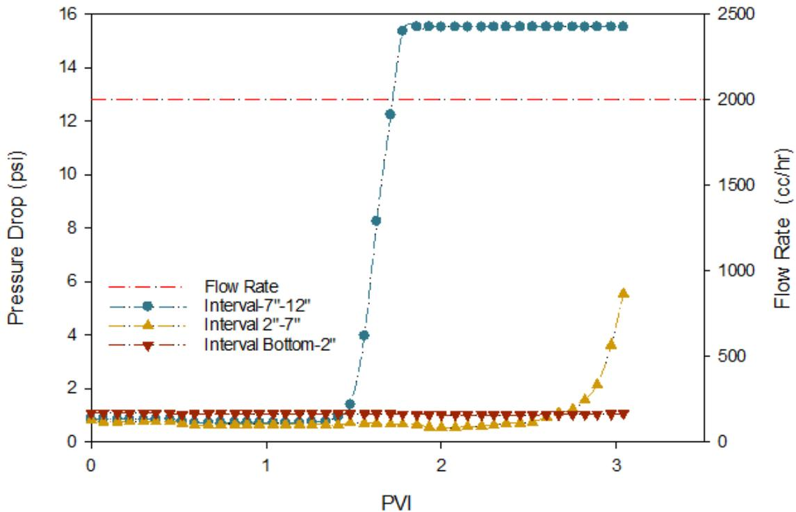
**Figure 3. 16:** Instant pressure drop variations at several intervals of the sand pack-Test No. 4.
