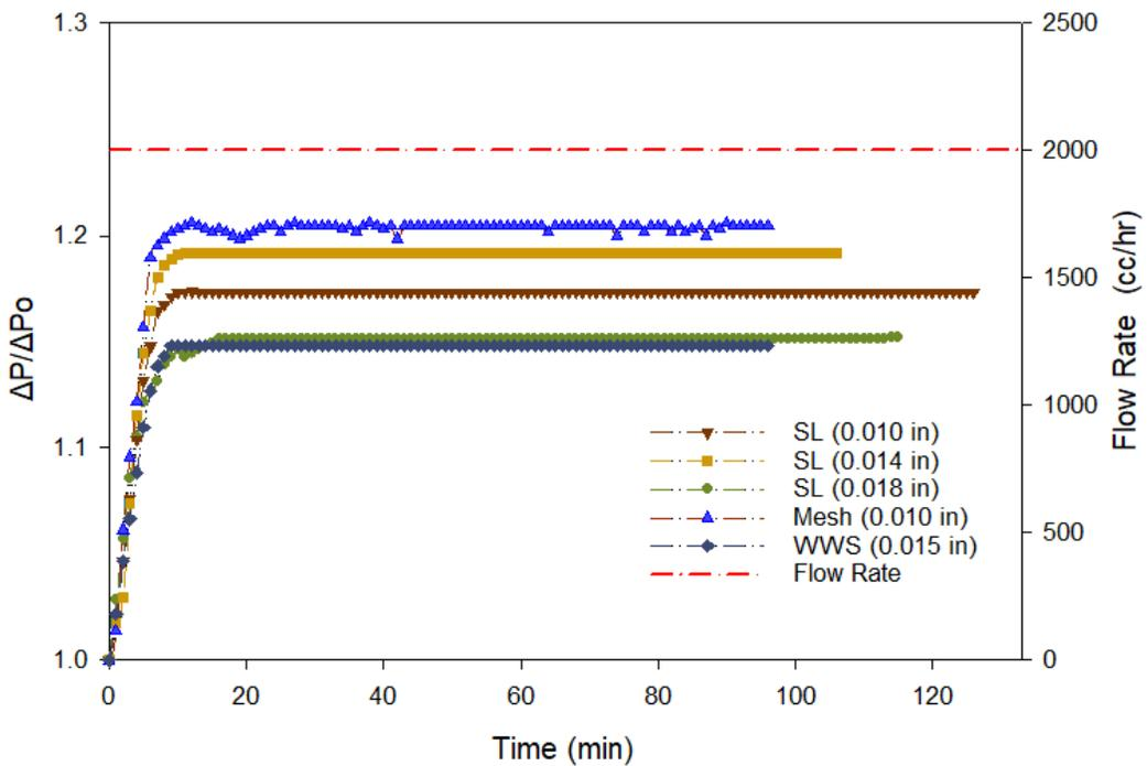
**Figure 4. 9:** Dimensionless pressure drop of the second 2.0" interval (away from the screen) for different sand screens, injecting 400 ppm brine.
