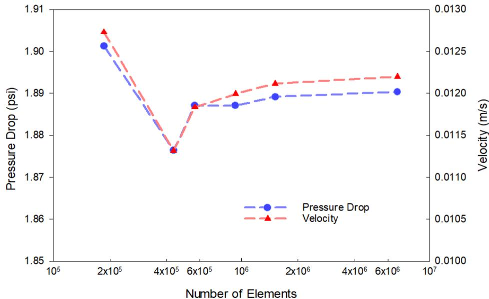
**Figure 4. 3:** The near-screen pressure drops and local velocities for different numerical mesh.
