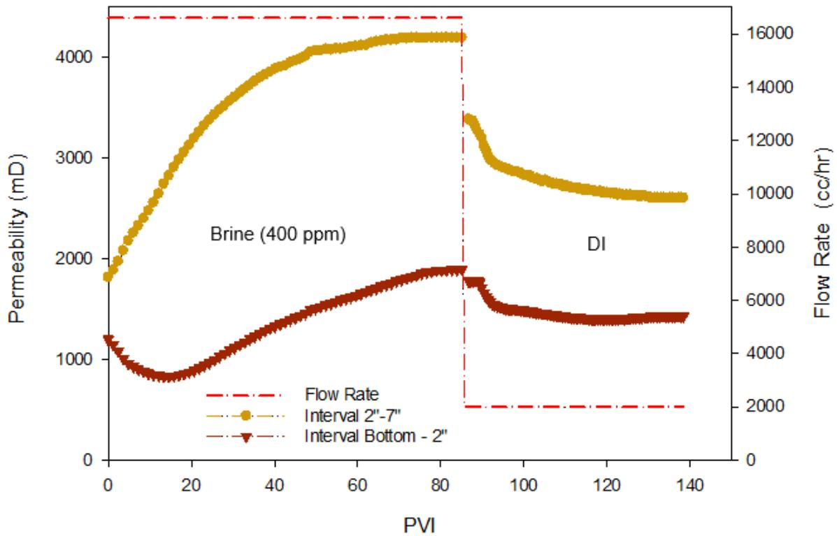
Figure 3. 18: Instant permeability variations at two intervals of the sand pack-Test No. 5.
