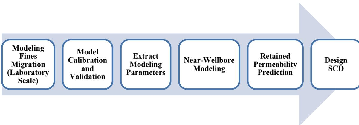
**Figure 2. 13:** Proposed workflow for SCD design accounting for transient behavior of the fines migration process.
