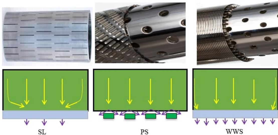
**Figure 1. 1: Different sand control screens with flowlines pattern schematics [24, 25].**
