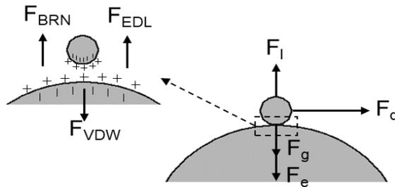
**Figure 2. 6:** Schematics of forces acting on fine particles attached to the grain surfaces.
