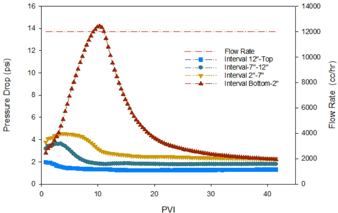
**Figure 3. 10:** Instant pressure drop variations at four intervals of the sand pack-Test No. 2.
