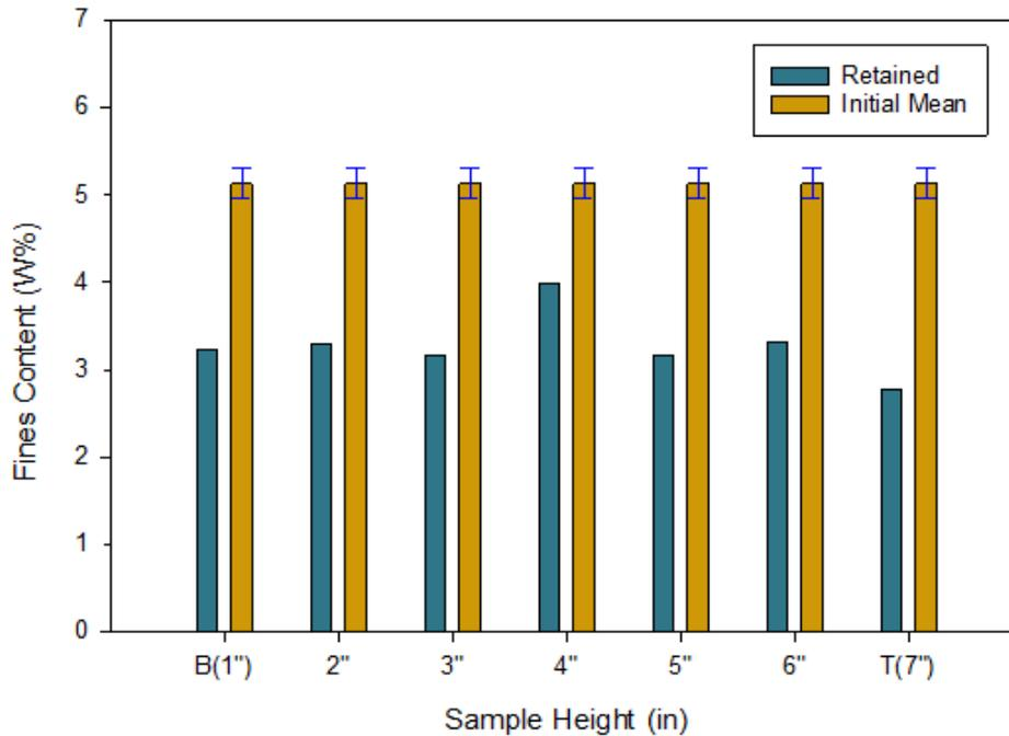
**Figure 3. 21:** Initial and retained fines content profile -Test No. 6.
