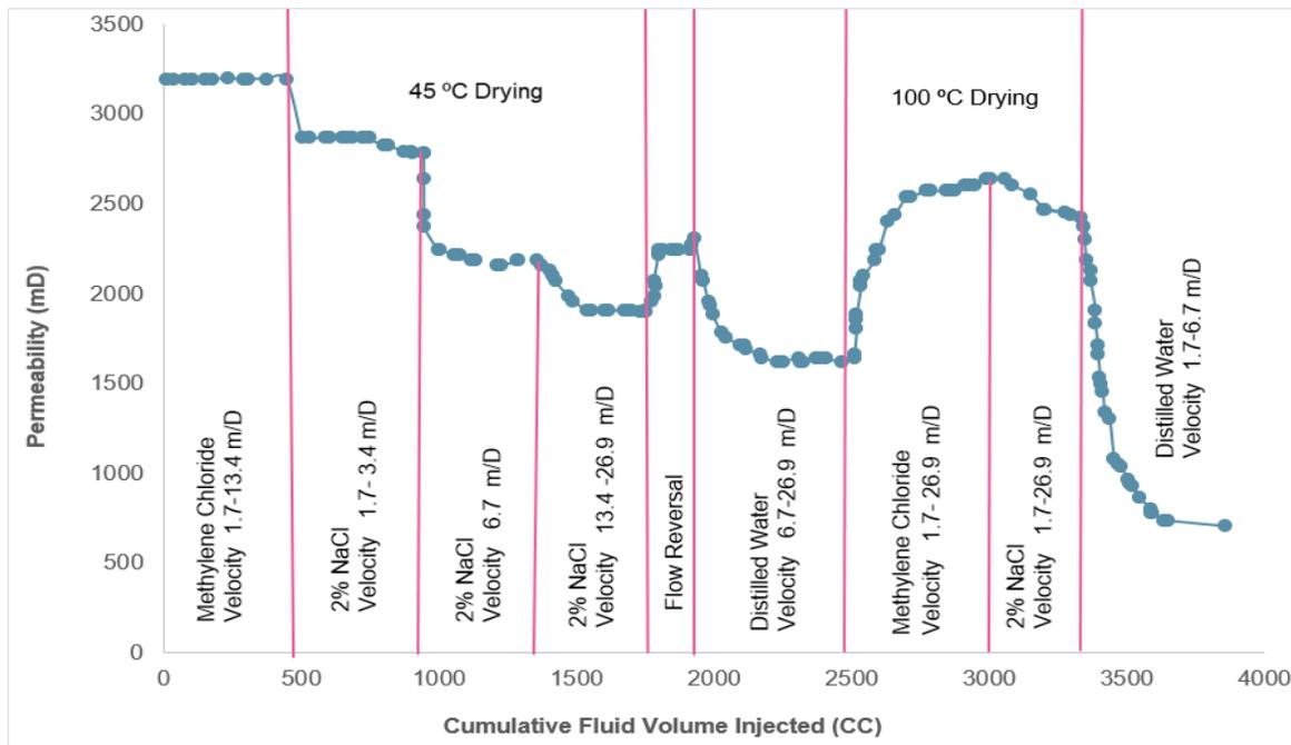
**Figure 2. 2:** Permeability variations of a preserved oil sand sample in different flow conditions [24].
