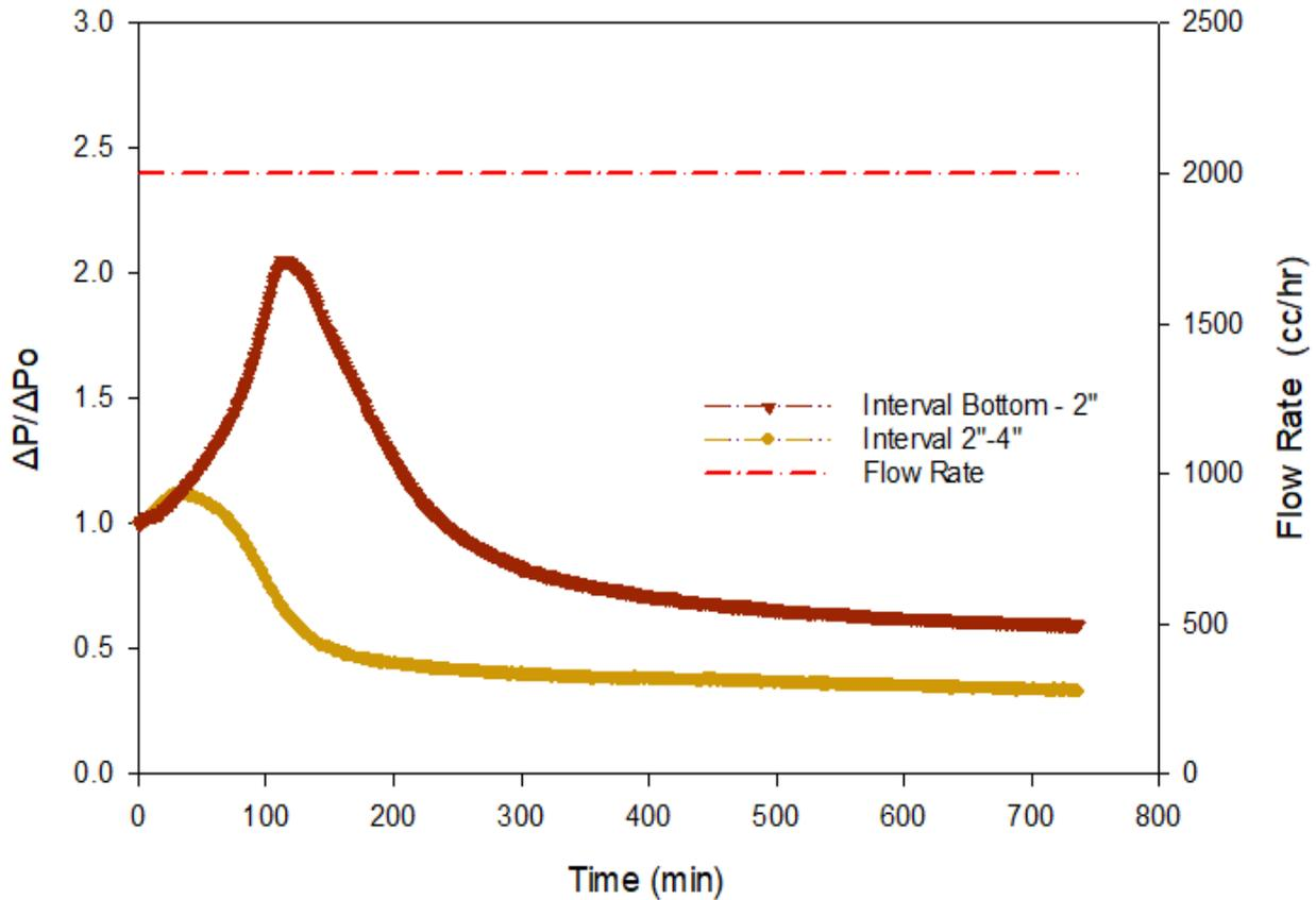
**Figure 4.5:** Dimensionless pressure drop variations for the first flow stage using SL 0.018" screen.
