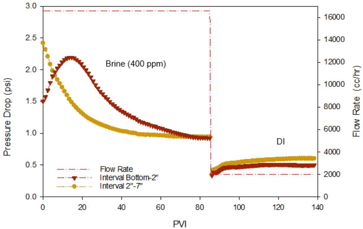
Figure 3. 17: Instant pressure drop variations at two intervals of the sand pack-Test No. 5.
