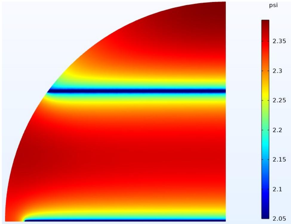
Figure 4A. 3: Pressure map solution near the slots before fines migration process, SL 0.010", 400 ppm brine flow top view.
