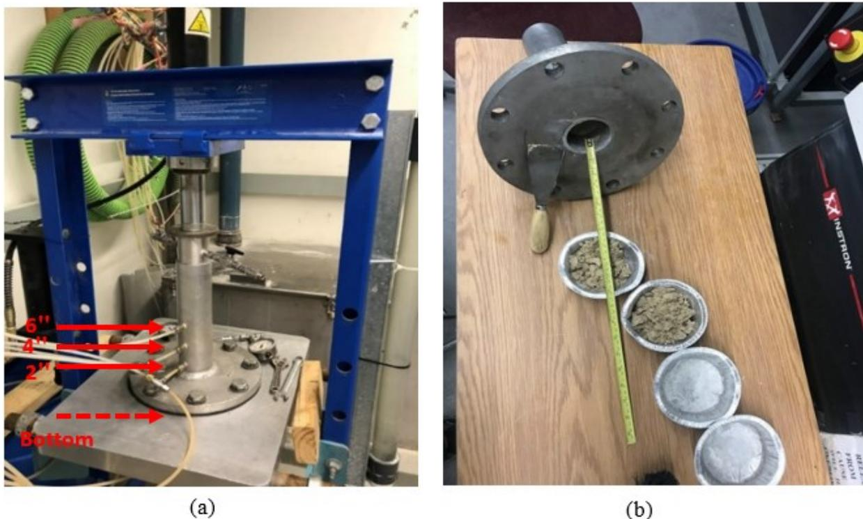
**Figure 4. 2:** (a) Photograph of the testing setup and sample cell, (b) taking 1-inch sand slices after the test.
