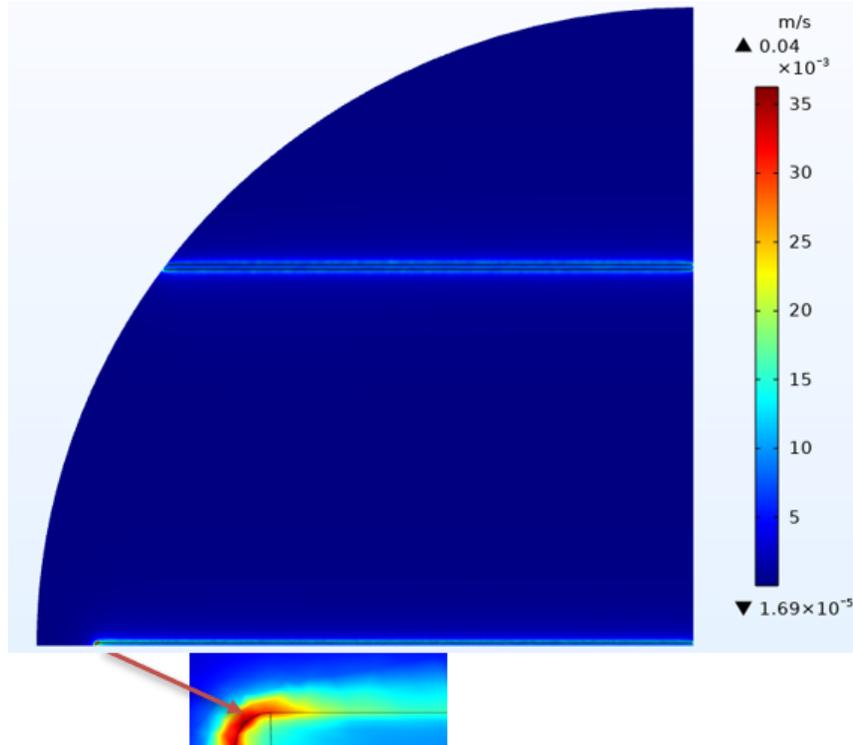
Figure 4A. 1: Darcy's velocity map near the slots, SL 0.010", top view.
