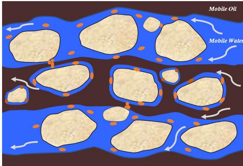
**Figure 2. 4:** Fines migration with the simultaneous oil and water flow (Modified after [3]).
