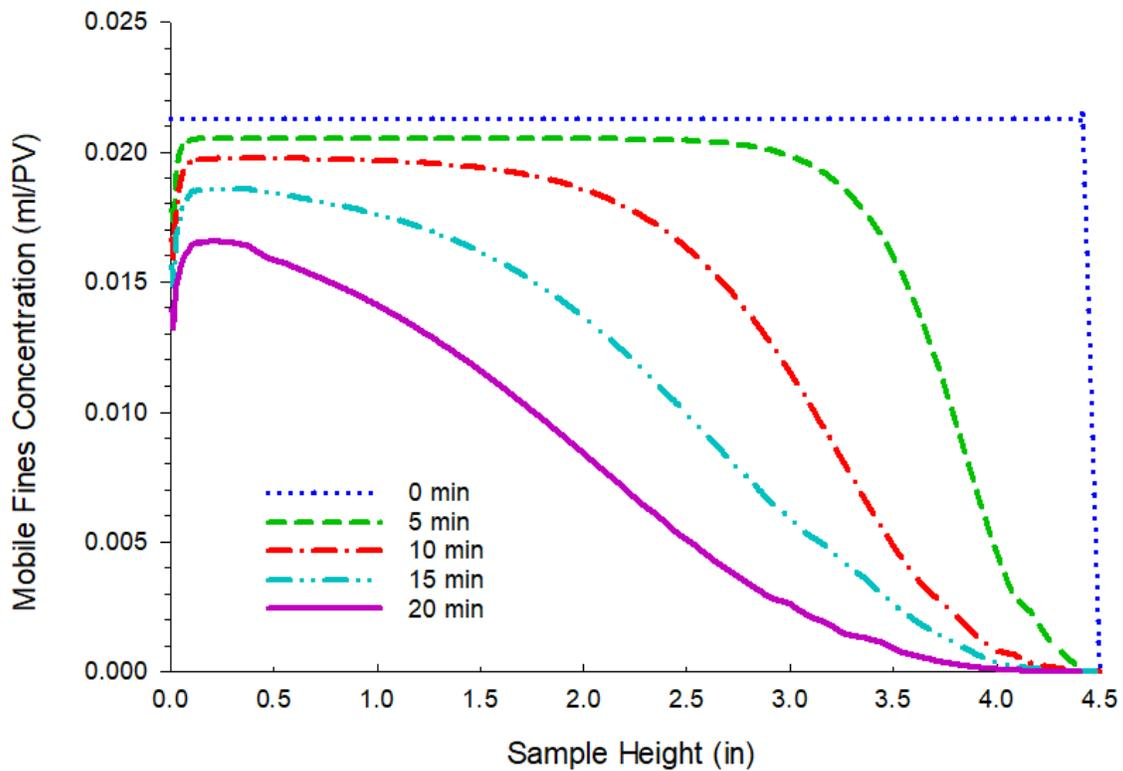
**Figure 4. 22:** Produced fines concentration profile for the test using SL 0.010" and injecting 400 ppm brine.
