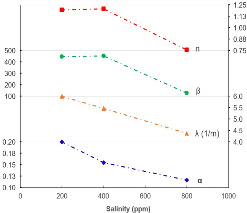
Figure 4. 25: Model parameters variations with brine salinity.
