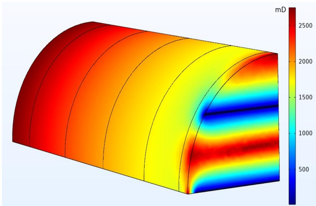
Figure 4A. 6: Permeability map at the end of the fines migration process, SL 0.010", 400 ppm brine flow.
