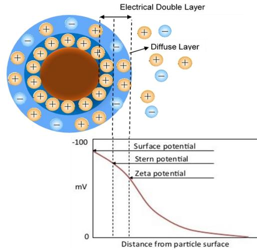
**Figure 2. 7:** Electrical double-layer demonstration.
