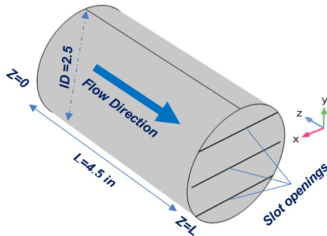
**Figure 4.12:** The schematic of the numerical model geometry.
