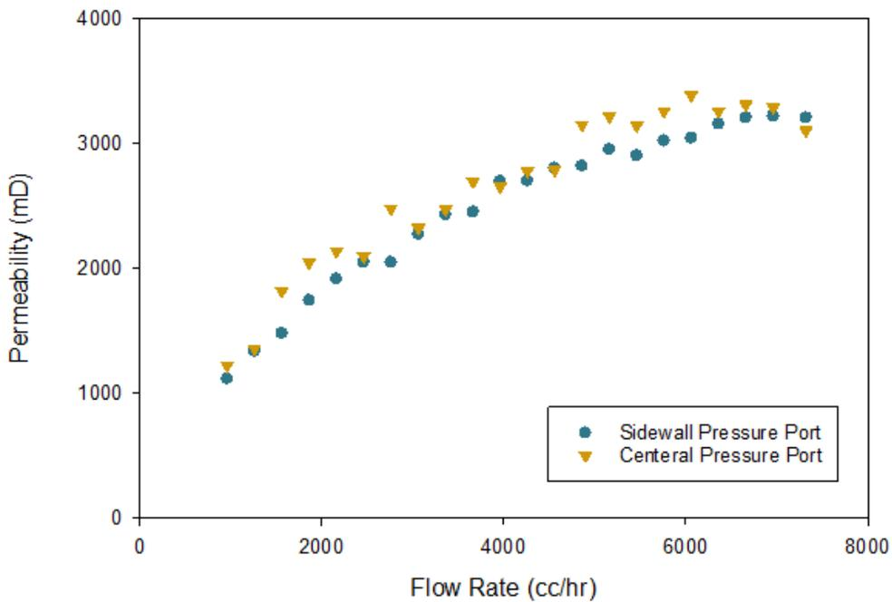
**Figure 3. 23:** Comparison of permeability variation with increasing flow rate based on the sidewall and central pressure transmitter ports.
