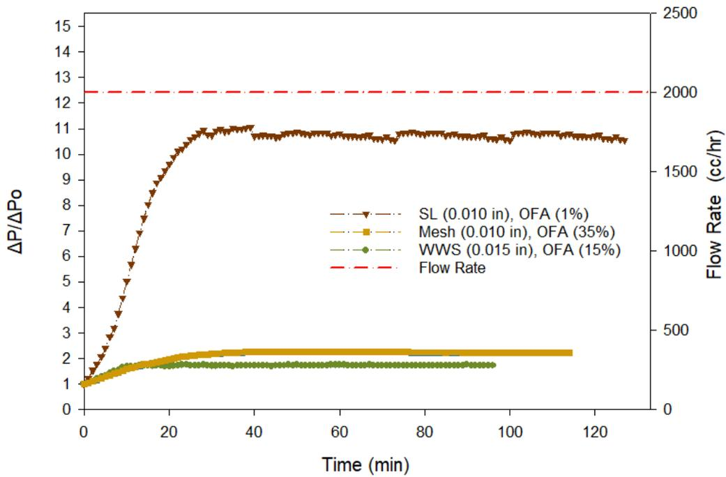
**Figure 4.8:** Near-screen dimensionless pressure drop for different sand screens, injecting 400 ppm brine.
