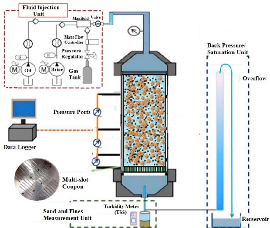
Figure 2. 10: Linear flow Large-Scale Sand Retention Test (SRT) setup [35, 56, 49, 53, 57, 58].
