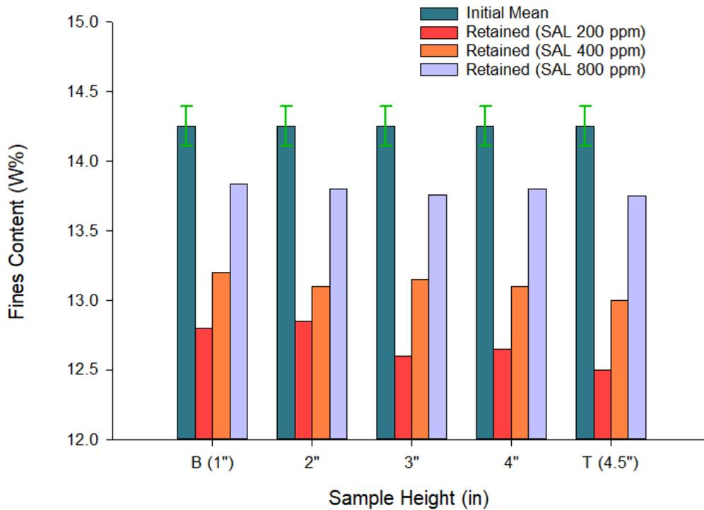
**Figure 4.11:** Initial and final fines content profile for the test using SL 0.010" and different brine salinity.
