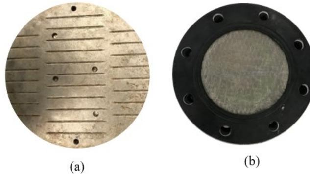
**Figure 3. 4:** (a) sand screen coupon (type: slotted liner; slot width: 0.01 inches; slot density: 42 SPC; opening: 1.3%)
