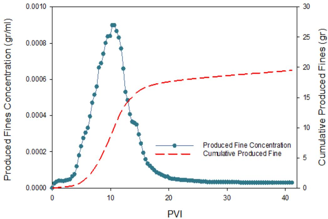
Figure 3. 12: Produced fines concentration versus injected pore volume -Test No. 2.
