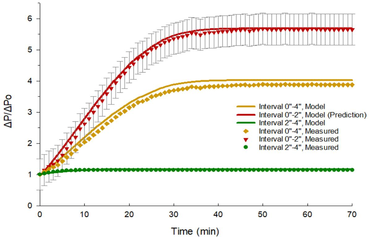
Figure 4. 17: The matched and predicted dimensionless pressure drops with error bars for the test using SL 0.018" and injecting 400 ppm brine.
