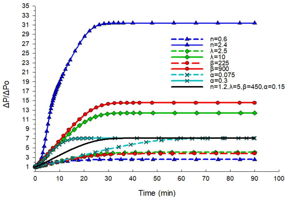
**Figure 4. 24:** Sensitivity of near-screen dimensionless pressure drop to doubling and halving the model parameters for the base case (solid line), using SL 0.014" and injecting 400 ppm brine.
