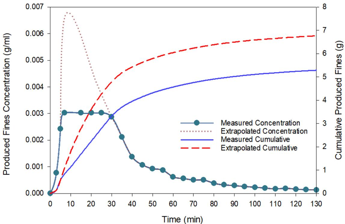
**Figure 4. 10:** Measured produced fines concentration for the test using SL 0.010" and injecting 400 ppm brine.
