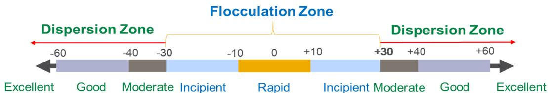
**Figure 2. 8:** Variation of the zeta potential and charged particle behavior.
