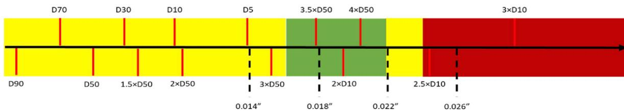
**Figure 2. 11:** Traffic light system for slotted liners with different aperture sizes (dashed lines), slot density 30, and flow rate <0.72 bbl/day/ft [71]
