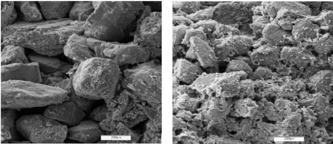
**Figure 4. 1:** Port throat plugging of oil sand core before (a) and after (b) steam injection (courtesy of SPE [18]).
