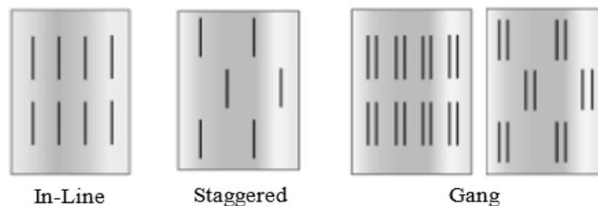
**Figure 2. 5:** Slotted liner with different slot patterns [69].
