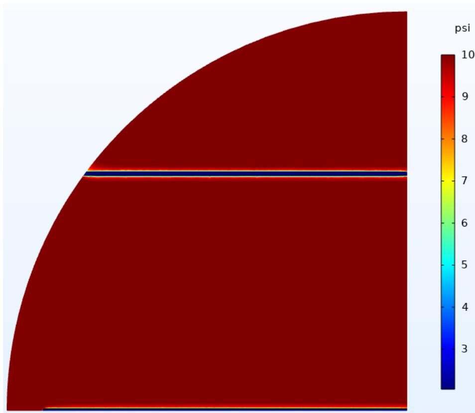
Figure 4A. 4: Pressure map solution near the slots after fines migration process, SL 0.010", 400 ppm brine flow, top view.
