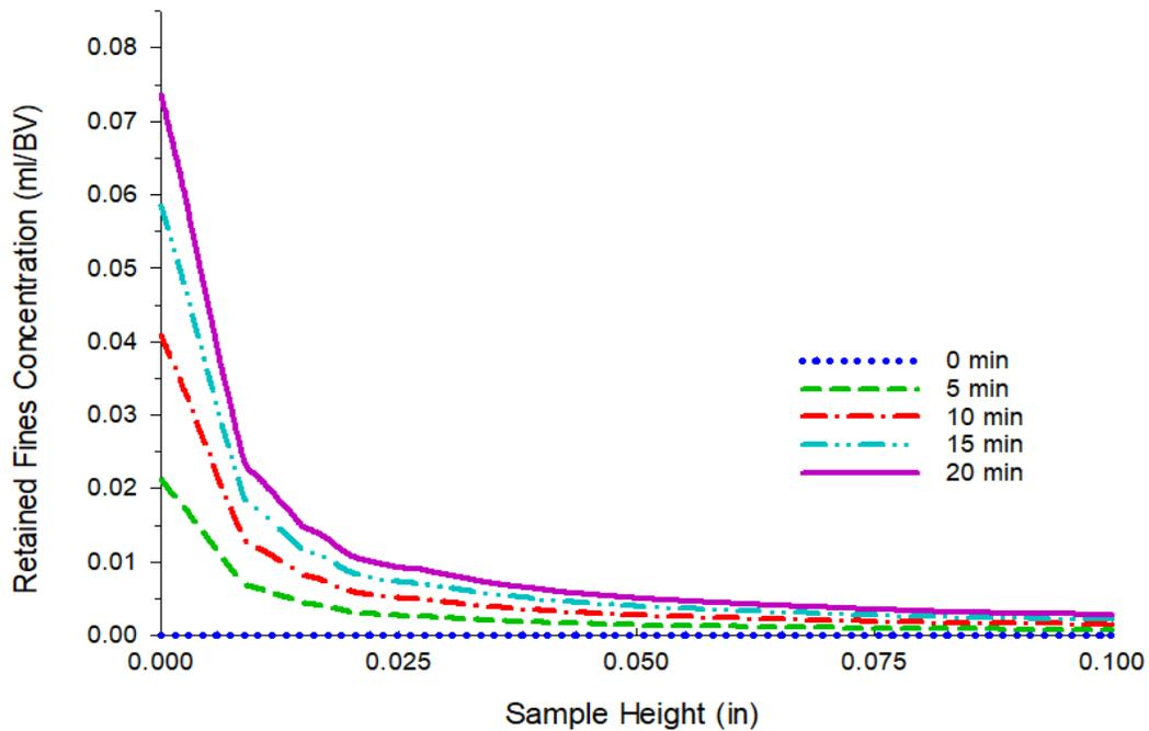
**Figure 4. 23:** Retained fines concentration profile (near-screen) for the test using SL 0.010", injecting 400 ppm brine.
