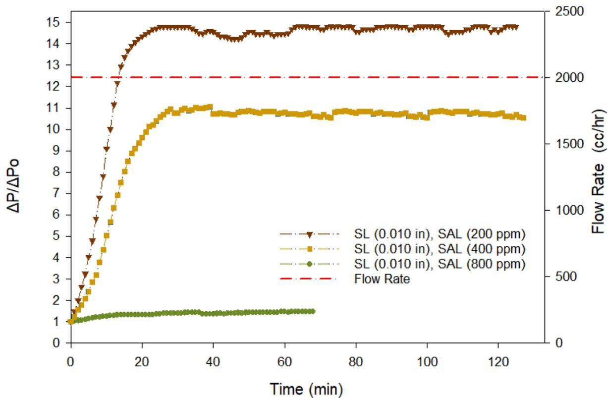
**Figure 4.7:** Near-screen dimensionless pressure drop variations for different brine salinity.
