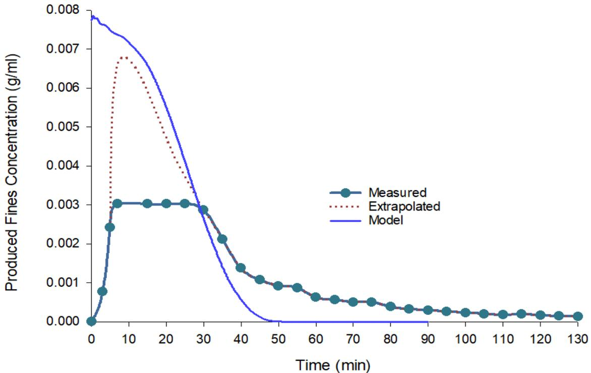
**Figure 4. 20:** The measured and calculated instant produced fines concentration for the test using SL 0.010" and injecting 400 ppm brine.
