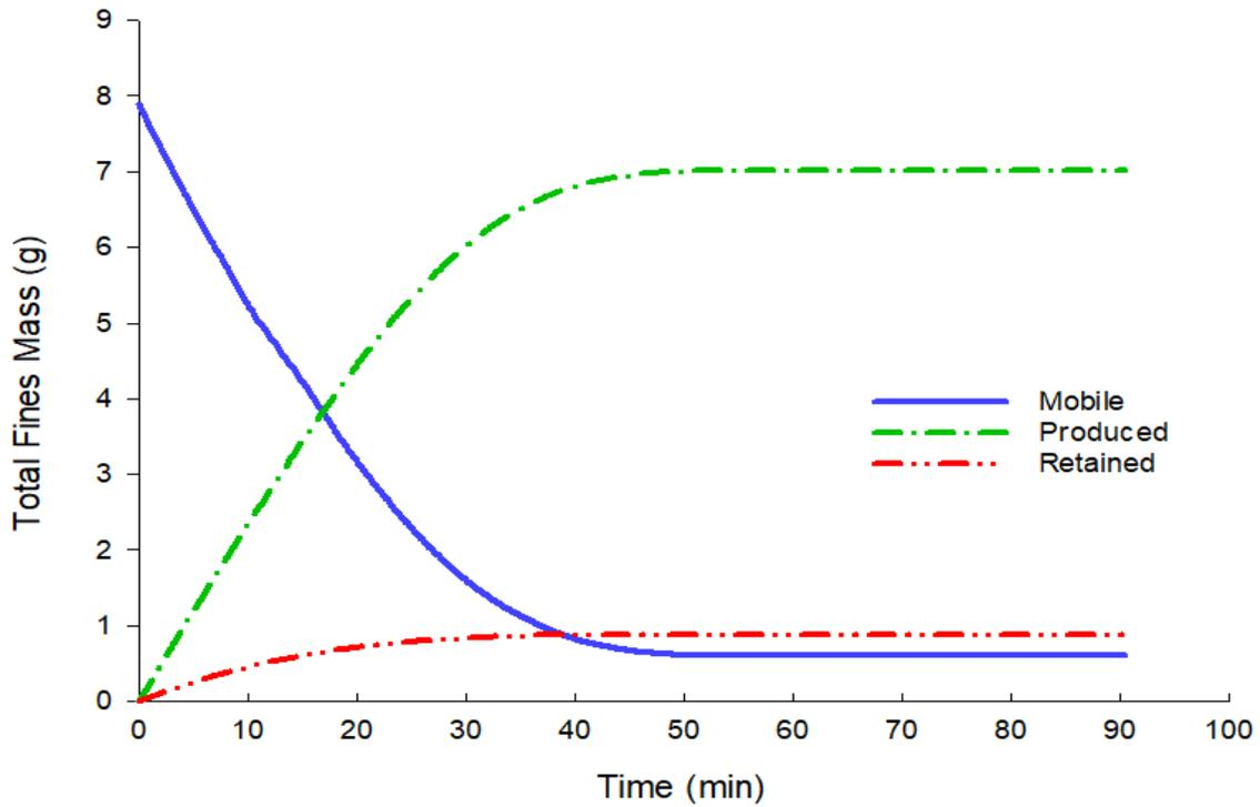
**Figure 4. 21:** Validity of mass conservation of migrating fine particles by the numerical model.
