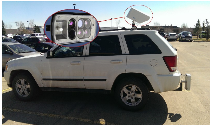
Figure 2. A mobile RWIS data collection unit equipped with spectral road surface temperature sensor
