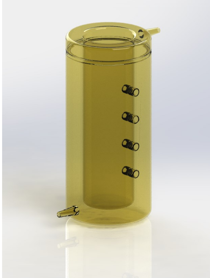
Figure 3-3: Rendering of CIST showing sampling ports and heating media attachments
