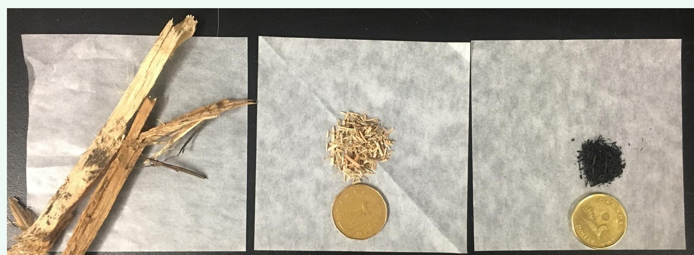
Figure 3: Wood is shredded to 1-2mm samples and then charred in the TGA
