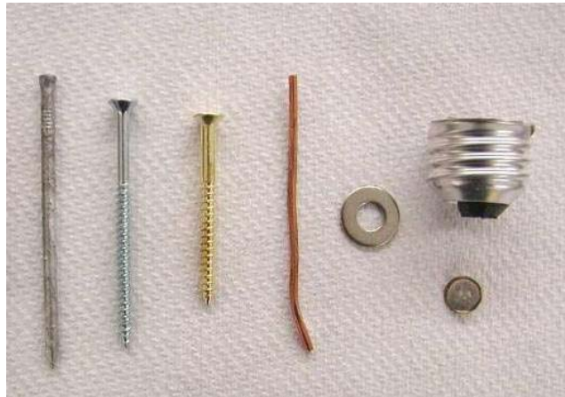
Figure 3-5 Contaminants used in this experiment (from left: galvanized nail, Zn-plated screw, brass screw, copper wire, stainless steel flat washer, incandescent light bulb tail with separated Al-thread and foot contact).
