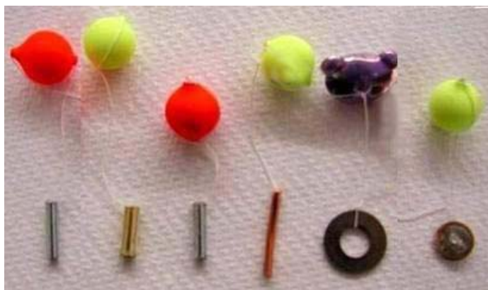
Figure 3-6 Specimens with indicator attached for the corrosion test (from left: galvanized nail, brass screw, Zn-plated screw, copper wire, stainless steel flat washer, light bulb tail foot contact).
