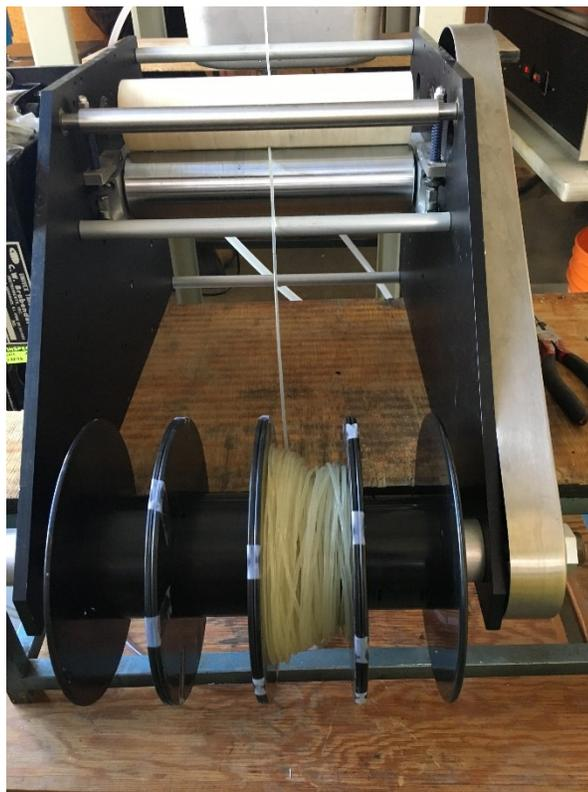
Figure 23: Drive system to wind filament
