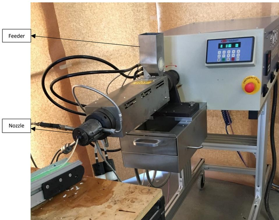
Figure 22: Brabender™ single screw extruder
