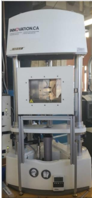
*Figure 26: Bose ElectroForce 3200 Series 3 test instrument*
