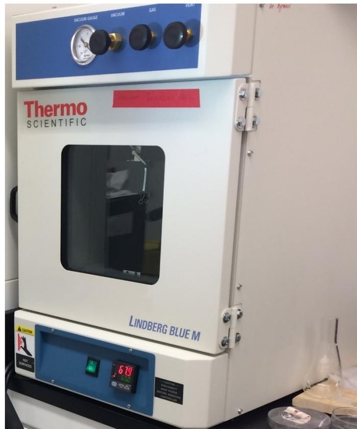
Figure 21: Vacuum Oven - Lindberg/Blue M from Thermo Fisher Scientific Inc.
