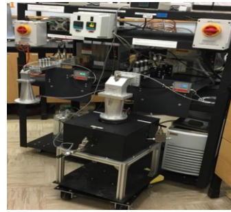
Assembled reactor vessel to the 2.45 GHz microwave unit
