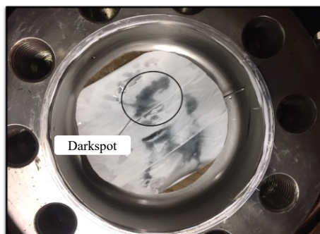
Figure 4-6. The darkspot on the thermal paper represents the regions where hotspots can be found in the reactor vessel.
