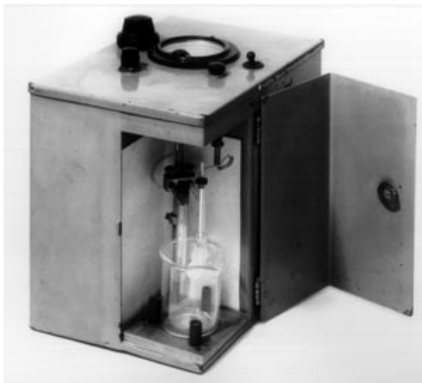
Figure 1.1 A picture of original model of pH meter constructed in 1934 by Arnold Beckman. Picture courtesy of Beckman Coulter, Inc.
