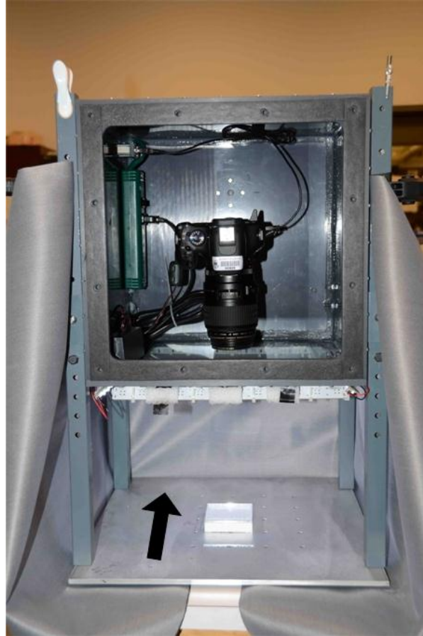
Figure 4-1: Camera setup and apparatus used to take high-definition video of UTLC plate during development. A black cloth is draped around the system to control lighting during the development. The camera is isolated from the development chamber in order to protect the camera lens from any potentially corrosive vapours. The arrow indicates the plate development direction.
