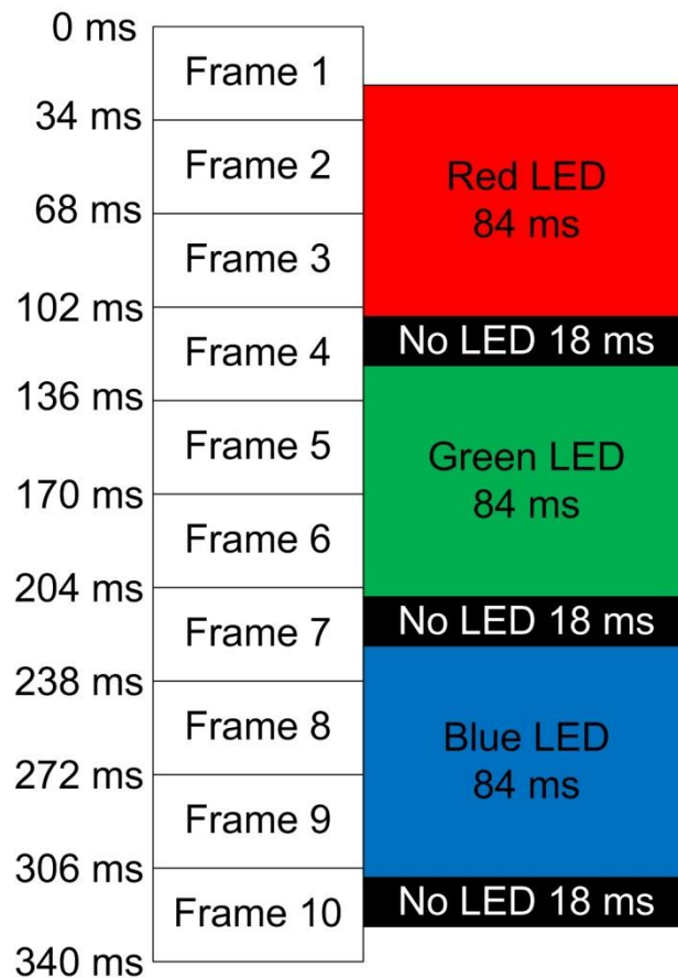
Figure 5-4: Schematic of the timing diagram used in the transmission mode video UTLC system. Over each complete period, it is ensured that at least one camera frame fully captures each LED color.
