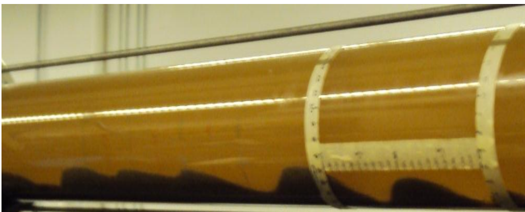
Figure 4.6a Bed form for slurry concentration greater than 1 vol%
