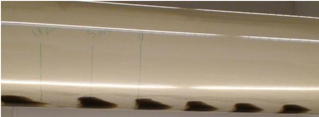
Figure 4.6b Bed form for slurry concentration of 0.5 vol%
