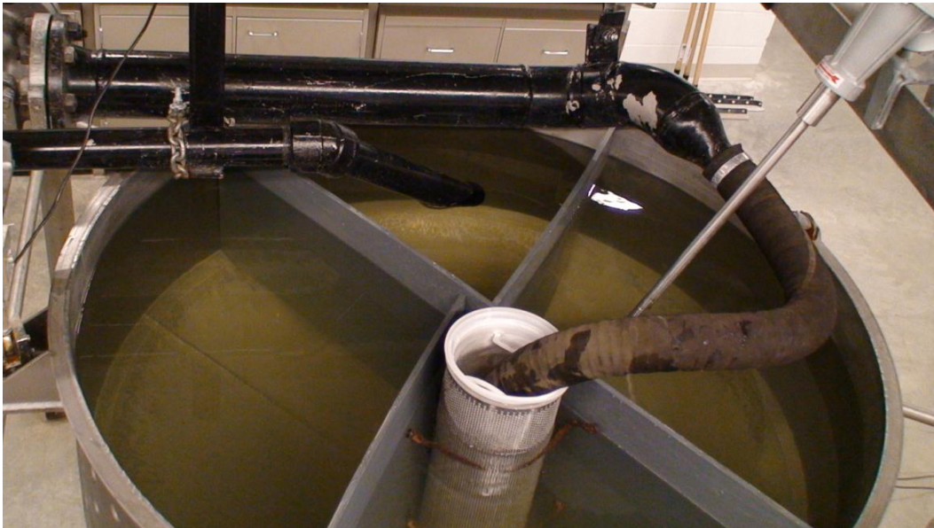
Figure 6.11 Micron-rated filter bag in the return line, to capture particles during circulation
