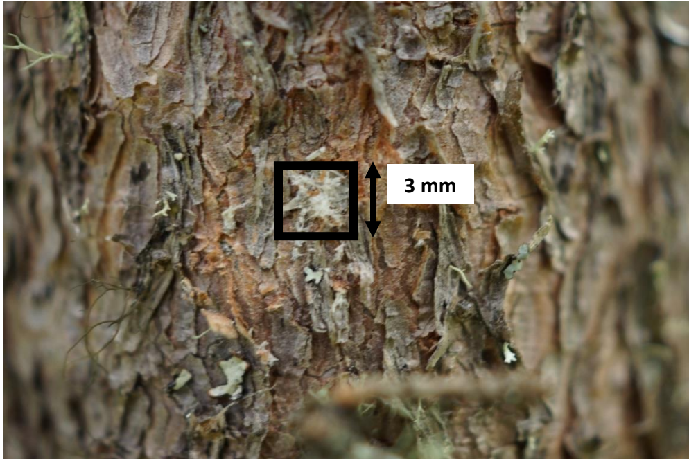
Plate 2.1: An example of the impact left by Resistograph drilling in white spruce. The only evidence left is a small borehole (3 mm) from the drill bit. As the bit is removed, the hole is filled with the drilling chaff. The borehole is highlighted by the black box.
