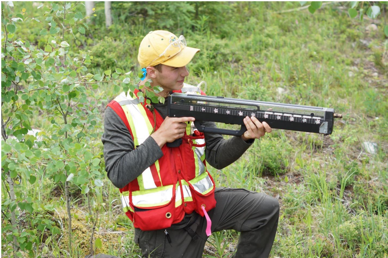
Plate 4.3: Jesse Shirton holding the Resistograph device in the typical fashion used for sampling in the present study. The end of the drill is held tightly against the tree stem and pressure is applied by leaning gently towards the tree to increase stability. The bottom handle may also be used to increase stability while sampling.
