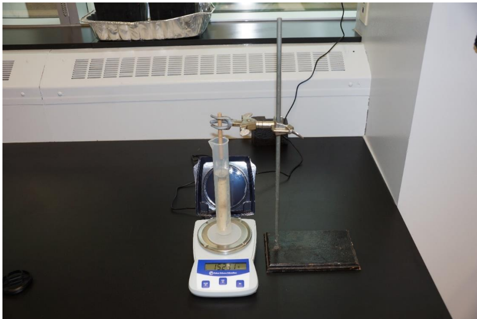
Plate 2.3: The apparatus used to measure the volume of a 5 mm increment core extracted from white spruce. The volume of the core (in ml) is equal to the mass of water displaced, which is 15.231 g in this example.
