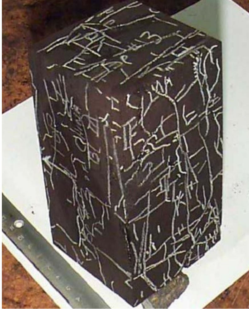
Figure 9. Outline of fractures inside of a coal seam (from Massarotto et al 2003).
