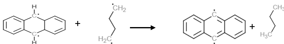
Figure 5-25. Hydrogen transfer from corresponding Clar aromatic \pi -sextets of anthracene to alkane radical.
