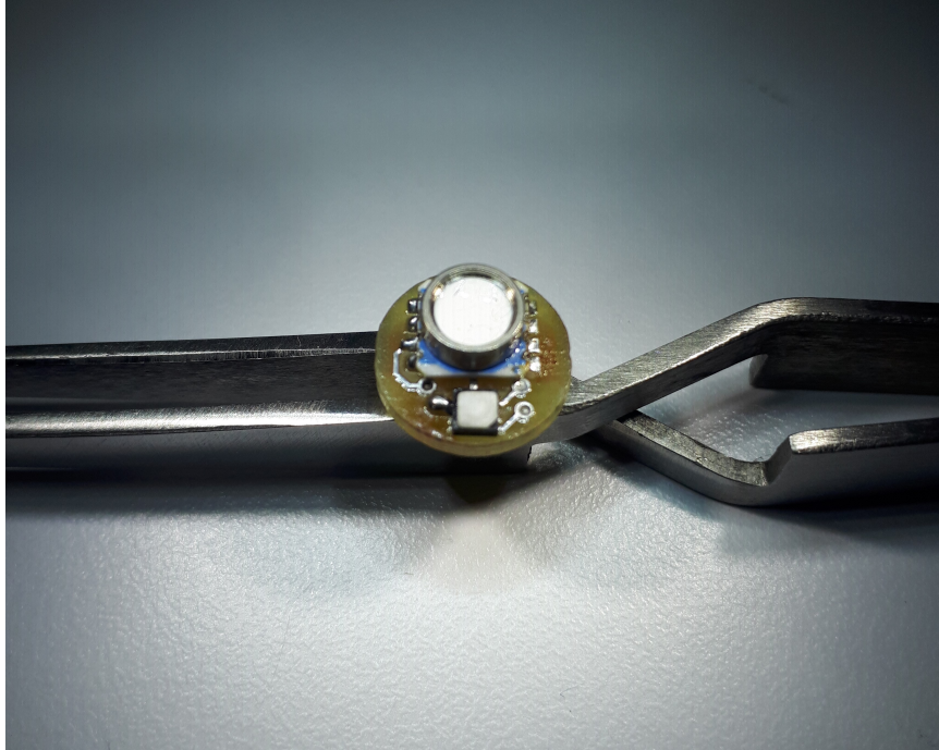
Figure A.1 – Prototype of custom PCB assembled with SHT35 and MS5803-01BA sensors
