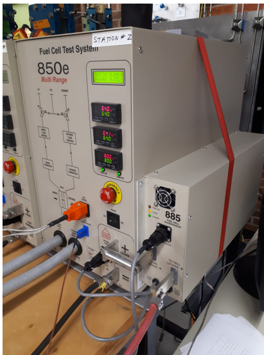
(a) Scribner 850e Fuel Cell Test Station
