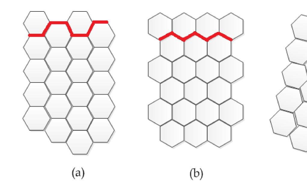
Figure 1) The different structural conformations of single-walled carbon nanotubes walls. The three structures are armchair (a), zigzag (b), and chiral (c). The red lines show the different orientates of the carbon bonds. Modified from: http://www.intechopen.com/source/html/16801/media/image2.png
