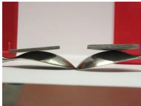
Figure 17: Comparison of two membranes: (Left) flat membrane prepared using flat bath steaming, and (Right) membrane prepared using stack steaming showing curvature
