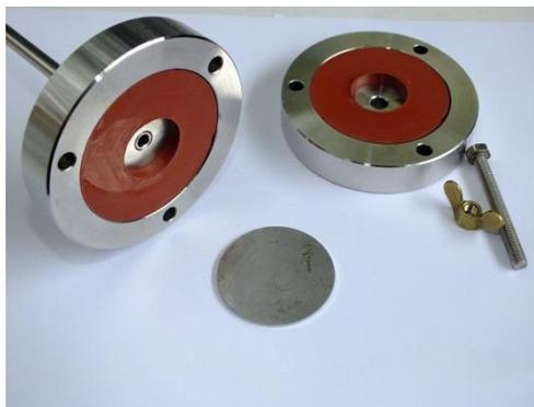
Figure 20: Air Leakage Test flange module with the stainless steel reference membrane
