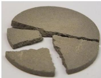
Figure 13: Cracked membrane prepared using autoclave steaming
