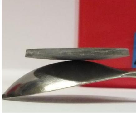
Figure 15: Curved membrane obtained using stack steaming
