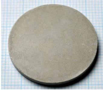
Figure 18: 33 wt% zeolite membrane after flat bath steaming
