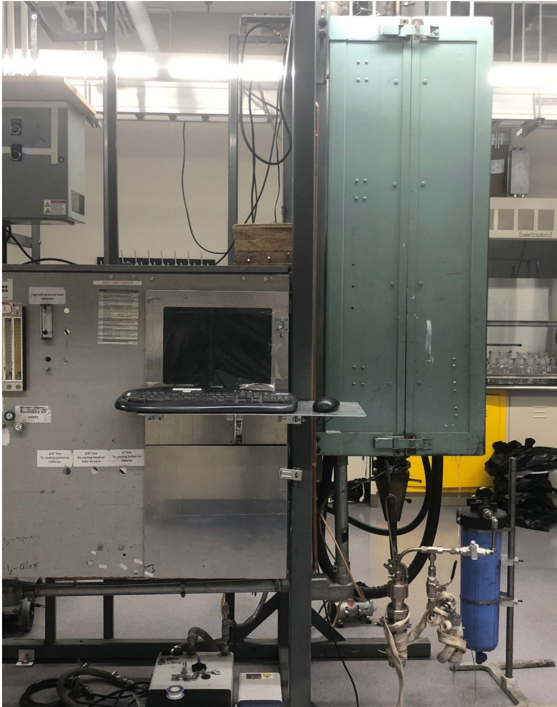
Figure 3.1 Electrically heated high temperature furnace
