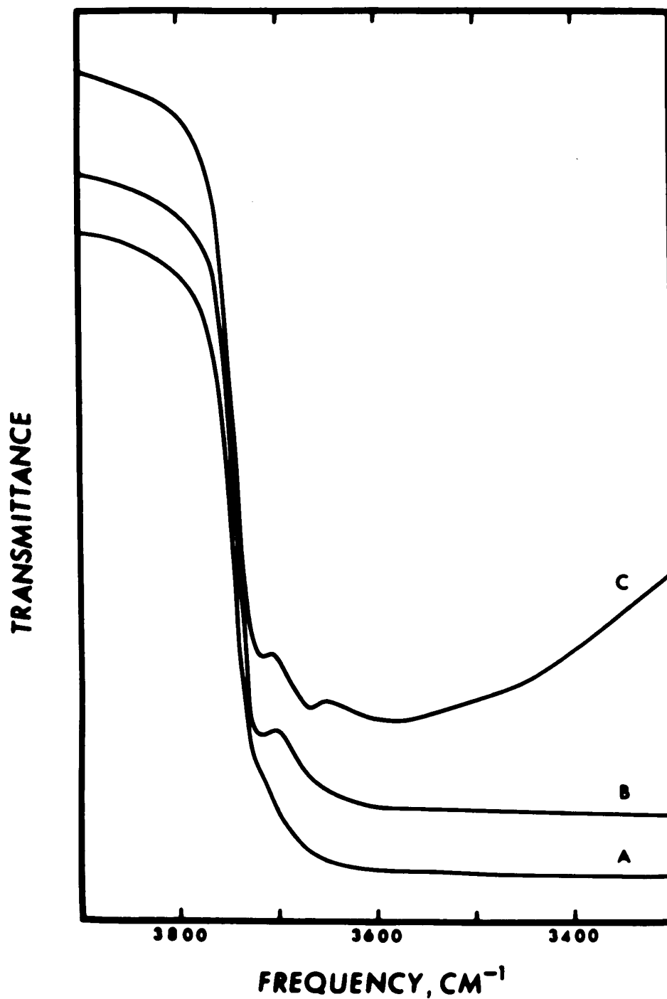
Figure 5-8. Spectra on the Degassing of \gamma -Alumina at Room Temperature over Varying Time Periods: A, 0.5 hr.; B, 4 hr.; C, 24 hr.
