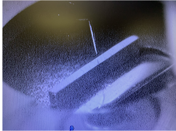
(b) Photograph of the STM tip over the freshly cleaved (110) face of the GaAs sample.
