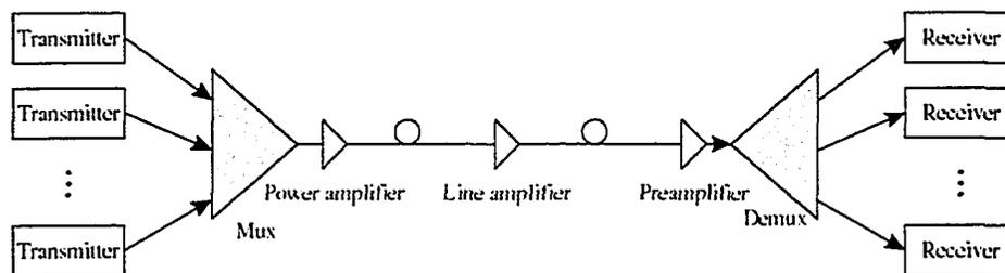
Figure 3.4. Point-to-point transport system. From [RaS02].
