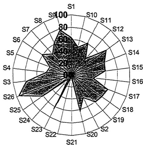
Figure 8.1. Used-to-total capacity ratio for each span,  $S$ , in the initial design (in percentages).
