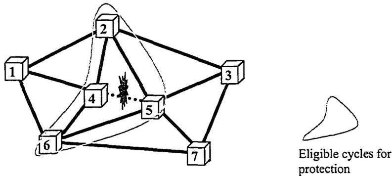
Figure 3.11.  $p$ -Cycles protection under a span failure.
