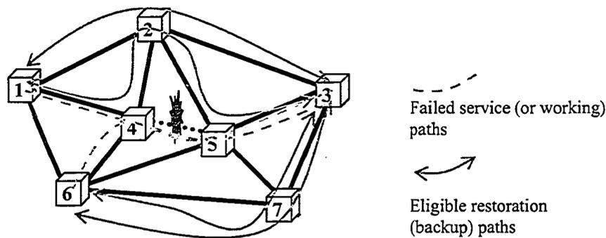
Figure 3.12. Illustration of the path restoration scheme.
