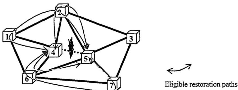
Figure 3.10. Span restoration under a span failure.
