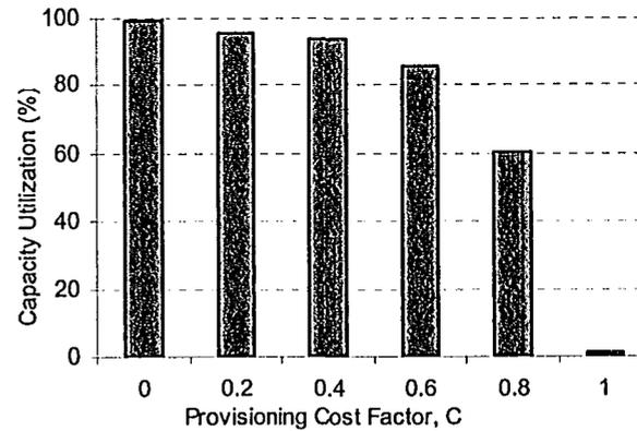
Figure 7.5. Total network capacity utilization by preferred demands as channel cost rises ( $\alpha = 1.2$ ).
