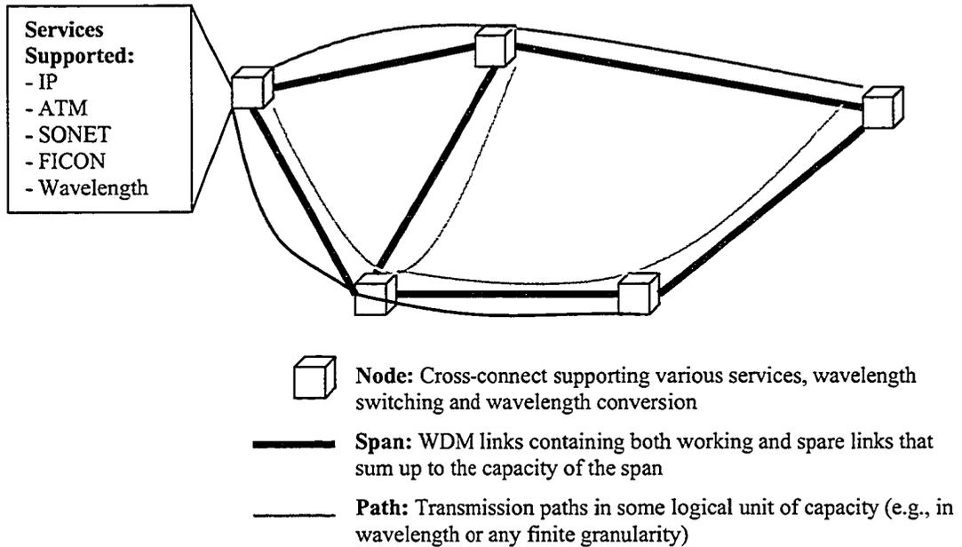
Figure 3.5. Generic survivable transport network model used in this thesis.
